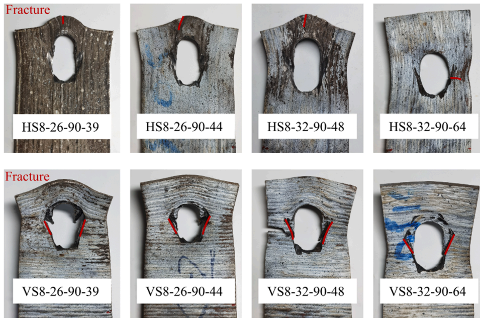
Fig. 21. Four pairs of specimens with different failure modes.
