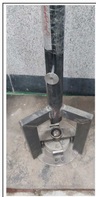
Figure 5. RDWI test device.
