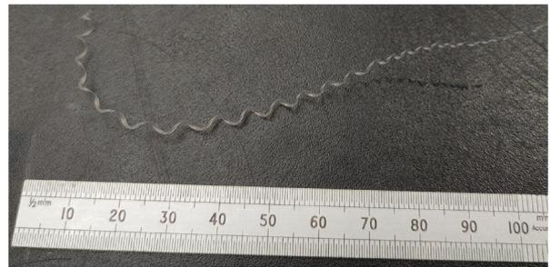
Figure 8. Post acetabular liner outer hemisphere roughing with LFV swarf.
