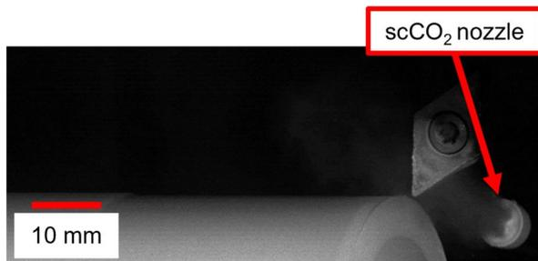
**Figure 15.** High-speed camera image of UHMWPE whilst using scCO<sub>2</sub>, prior to the first cut.
