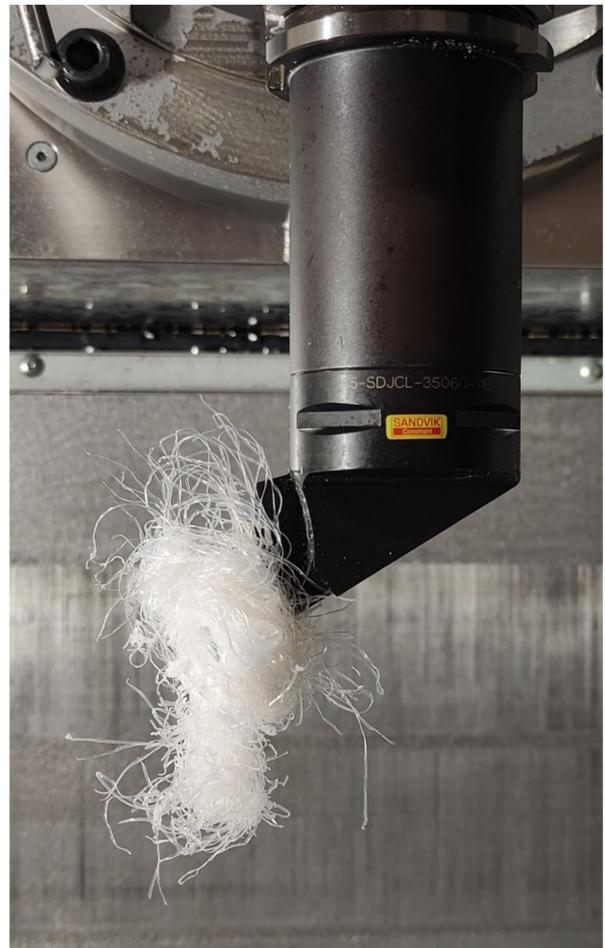
**Figure 5.** UHMWPE swarf melted to the insert post hemisphere roughing.
