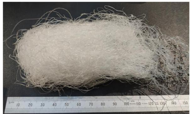
**Figure 6.** Post acetabular liner outer hemisphere roughing without LFV swarf.
