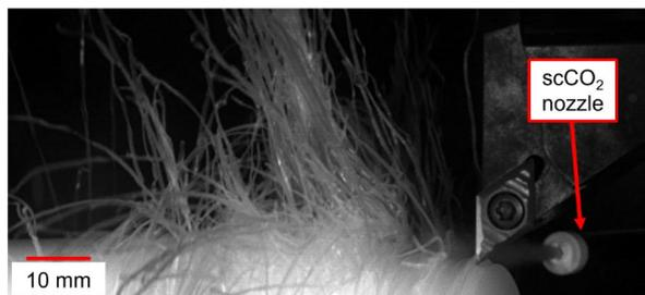
**Figure 17.** High-speed camera image of UHMWPE whilst using scCO<sub>2</sub> near the centre of the hemisphere.
