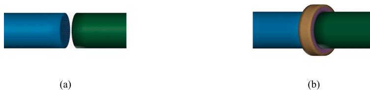
Fig. 26. LS-DYNA zoom-in on modelling for (a) the unconfined SHPB setup, and (b) the confined SHPB setup.
