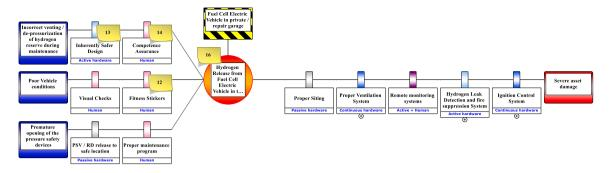
Fig. 8. Hydrogen vehicle private/repair garage bowtie diagram.
