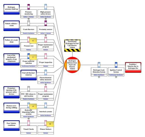
Fig. 6. Hydrogen fuel cell vehicle bowtie diagram.
