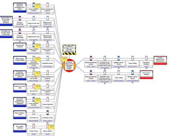
Fig. 4. HRS bowtie diagram.
