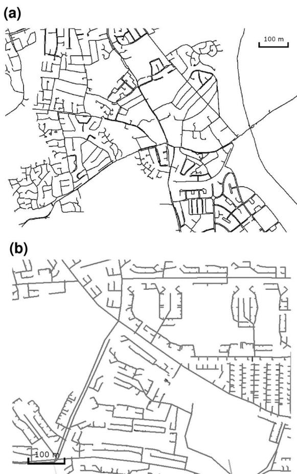
**FIGURE 1** | Examples of (a) water distribution and (b) wastewater pipe networks in towns in the UK.
