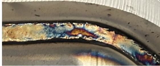
Figure 11: A corner of the workpiece showing significantly improved welding quality after system re-calibration.
