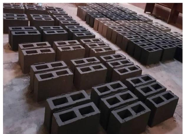
Figure 5. Freshly prepared hollow sandcrete blocks.
