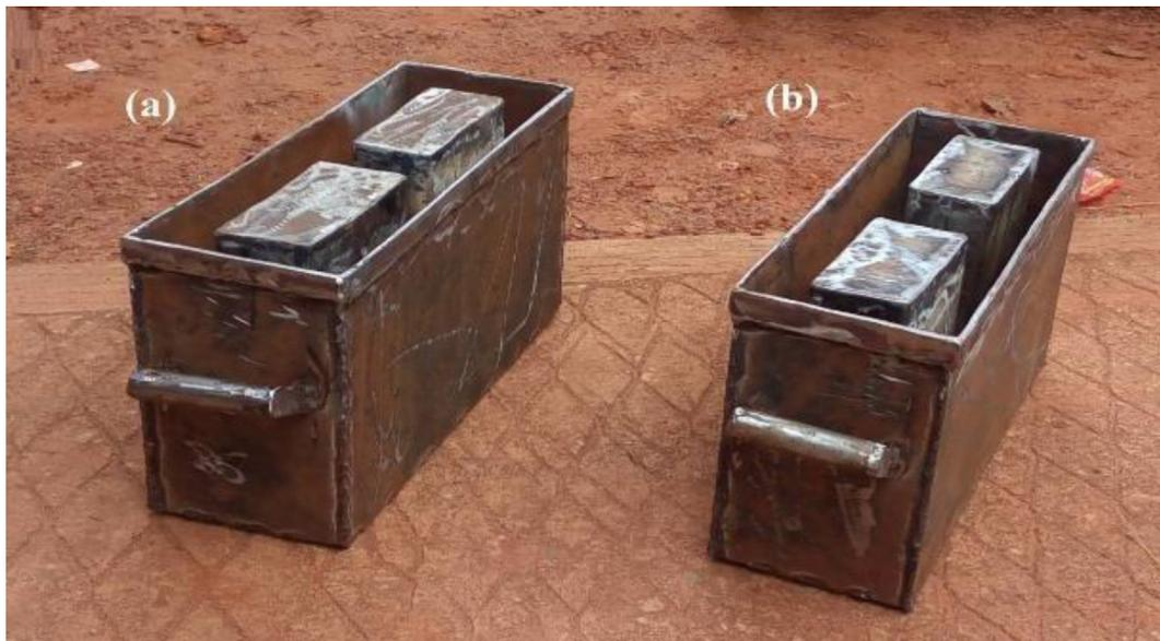
Figure 4. Fabricated moulds: (a) mould with end-web to centre-web ratio of 1:1; (b) mould with end-web to centre-web ratio of 1:2.
