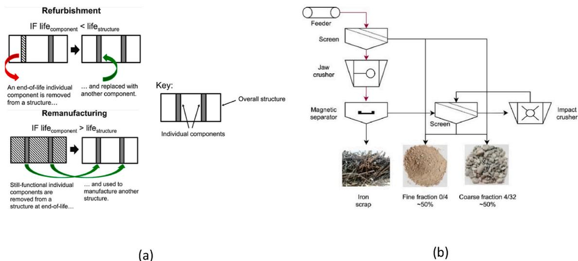
Fig. 1. Circular end-of-life management options for concrete structures: (a) Reutilisation options, reproduced from Ref. [3] (b) Recycling option, reproduced from Ref. [43].
