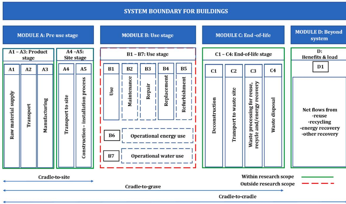
Fig. 4. System boundary considered for the remanufacture to demolition circularity scenarios for the building case scenario, according to BS EN 15978.
