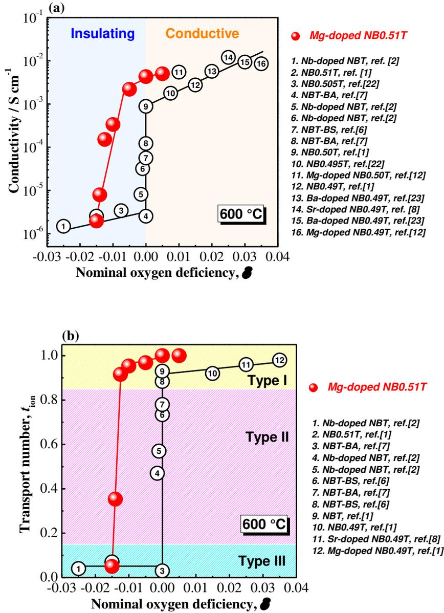
Fig.9 (a) Bulk conductivity,  $\sigma_b$  and (b) oxide-ion transport number,  $t_{ion}$  of NBT-based materials as a function of nominal oxygen deficiency,  $\delta$ . The solid spheres represent the data for Mg-doped NB<sub>0.51</sub>T in this work, and the open circles are data from literature.
