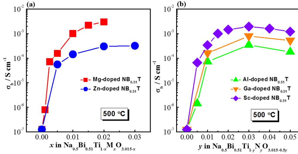
Fig.8 Bulk conductivity,  $\sigma_b$ , for  $Na_{0.5}Bi_{0.51}TiO_{3.015}$  with various acceptor dopants and doping levels: (a) divalent dopants  $Mg^{2+}$  and  $Zn^{2+}$ ; (b) trivalent dopants  $Al^{3+}$ ,  $Ga^{3+}$  and  $Sc^{3+}$ .
