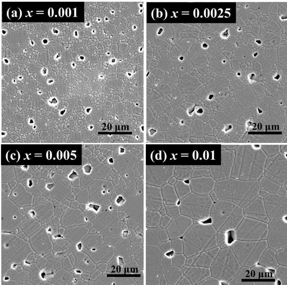
Fig.2 SEM micrographs of thermally-etched surfaces of  $\text{Na}_{0.5}\text{Bi}_{0.51}\text{Ti}_{1-x}\text{Mg}_x\text{O}_{3.015-x}$  ceramics. (a)  $x = 0.001$ ; (b)  $x = 0.0025$ ; (c)  $x = 0.005$ ; (d)  $x = 0.01$ .
