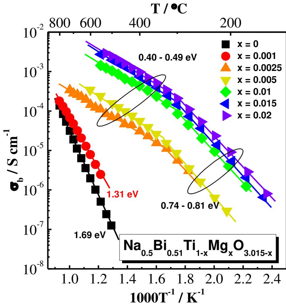
Fig.5 Arrhenius plot for bulk conductivity,  $\sigma_b$ , of  $\text{Na}_{0.5}\text{Bi}_{0.51}\text{Ti}_{1-x}\text{Mg}_x\text{O}_{3.015-x}$  ( $x = 0, 0.001, 0.0025, 0.005, 0.01, 0.015$  and  $0.02$ ) ceramics measured in air. Numbers in eV are the activation energies associated with bulk conduction.
