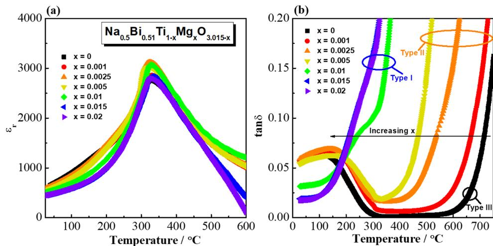
Fig.7 Dielectric spectroscopy for  $\text{Na}_{0.5}\text{Bi}_{0.51}\text{Ti}_{1-x}\text{Mg}_x\text{O}_{3.015-x}$  ( $x = 0, 0.001, 0.0025, 0.005, 0.01, 0.015$  and  $0.02$ ) ceramics: (a) permittivity at 1 MHz versus temperature and (b) dielectric loss,  $\tan \delta$ , (1 MHz) versus temperature.
