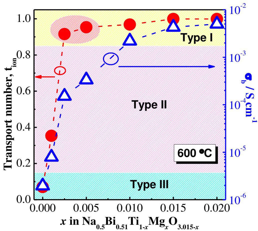
Fig. 6 Oxygen-ion transport number,  $t_{\text{ion}}$ , and bulk conductivity,  $\sigma_b$ , at 600 °C versus  $x$ .
