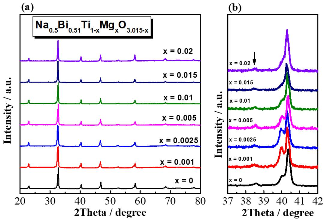
Fig.1 (a) Room temperature XRD patterns of  $\text{Na}_{0.5}\text{Bi}_{0.51}\text{Ti}_{1-x}\text{Mg}_x\text{O}_{3.015-x}$  ( $x = 0, 0.001, 0.0025, 0.005, 0.01, 0.015$  and  $0.02$ ) ceramics and (b) an expanded view of the  $2\theta$  range between  $37$  and  $42^\circ$  showing the superlattice reflection of the rhombohedral structure as indicated by the arrow.
