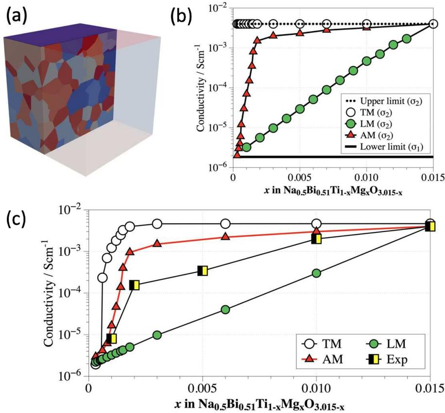
Fig.13 (a) A 3D geometric model for finite element simulations; (b) the relationship between Mg content, and the upper and lower conductivity limits. The lower limit is assigned to  $\sigma_1$ , the upper limit is modified and assigned to  $\sigma_2$  through a TM (threshold model), LM (linear model) and AM (area model). (c) Calculated dc conductivity versus  $x$  using three separate conductivity profile models TM, LM and AM, in comparison with experimental results (Exp).
