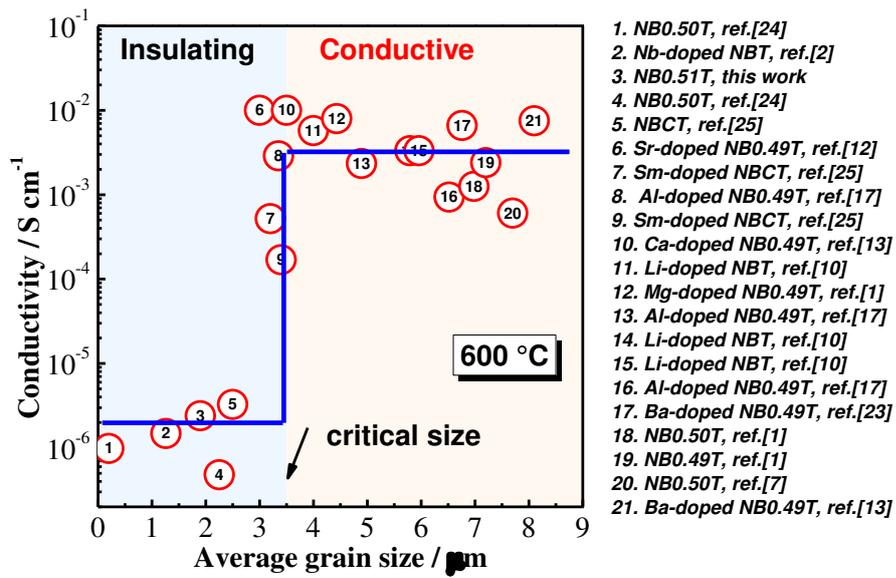
Fig.10 Conductivity-average grain size relationship of nonstoichiometric and doped NBT ceramics.
