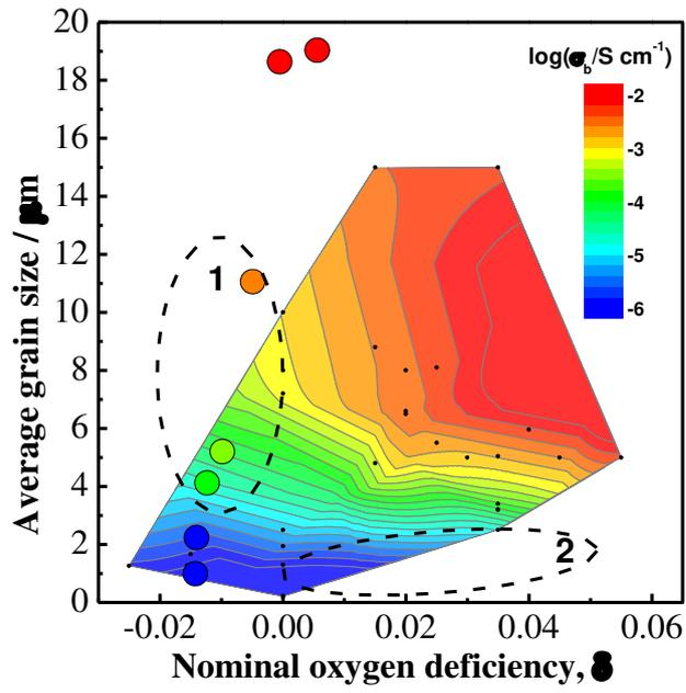
Fig.11 A contour map showing the dependence of bulk conductivity (at 600 °C) on nominal oxygen deficiency and average grain size. The contour map is plotted based on data collected from references listed in Figs.9 and 10. The filled circles are experimental data from this work.
