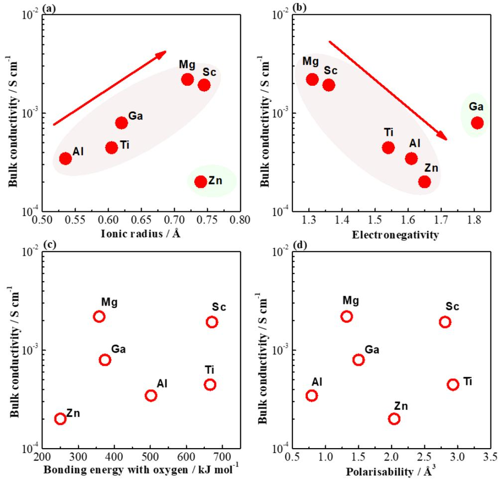
Fig.14 Bulk conductivity as a function of (a) ionic radius, (b) electronegativity, (c) bonding energy with oxygen and (d) polarisability of dopant ions.
