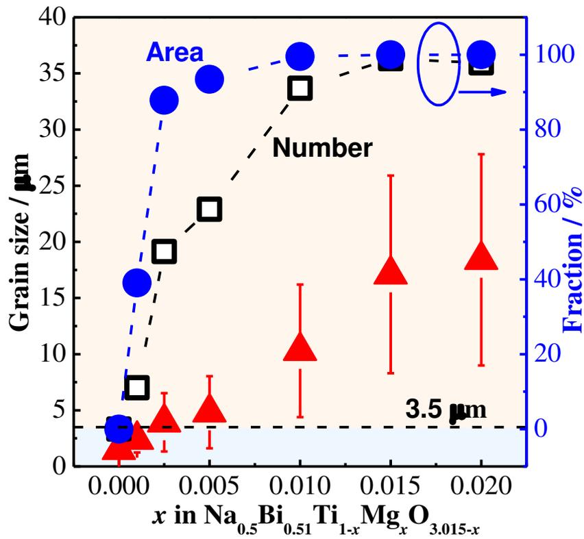
Fig.12 Average grain size (filled triangles), number (open squares) and area (filled cycles) fractions of large grains ( $d > 3.5 \mu\text{m}$ ) as a function of  $x$ . The horizontal dash line represents the critical grain size for the insulating-conductive transition.
