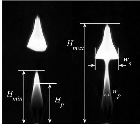
Fig. 4 Definitions of flame dimensional parameters.
