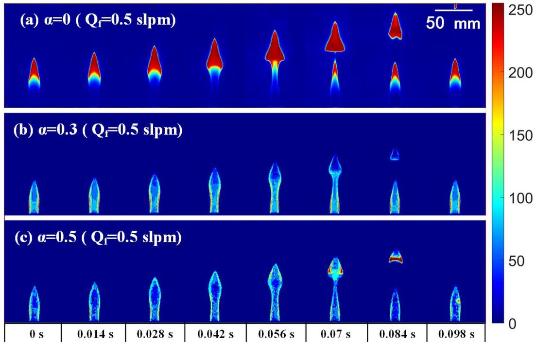
Fig. 13 The variation of flame brightness at various ammonia ratios over time.
