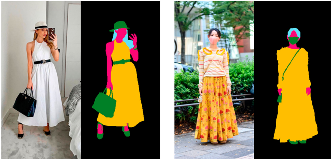
Figure 1. Two example images from the training set showing the corresponding annotated images that were produced for training purposes. The colour code used was black (null), green (shoes and accessories), cyan (hair), magenta (skin) and yellow (clothing).
