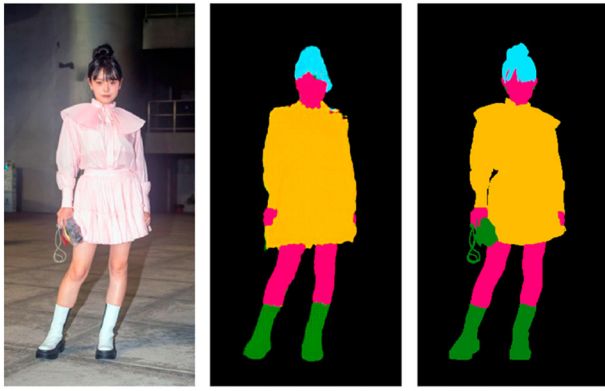
Figure 4. Example performance for the network trained for 40 epochs on input image (left). The output image (middle) shows the output of the network and 97% of the pixels are correctly classified compared with the ground truth data (right).
