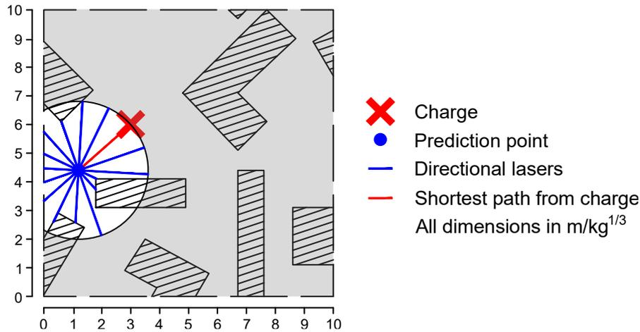
**Figure 2.** Zone of influence for a given prediction point. Drawn as a circle with radius equal to the shortest path distance from the charge.
