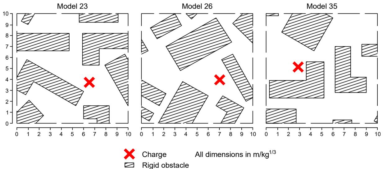
**Figure 4.** Three example domains used in the training dataset.
