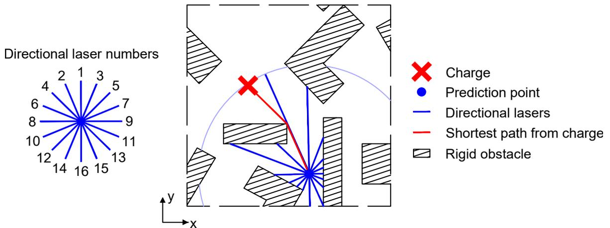
**Figure 1.** Summary of directional inputs to the Machine Learning model.
