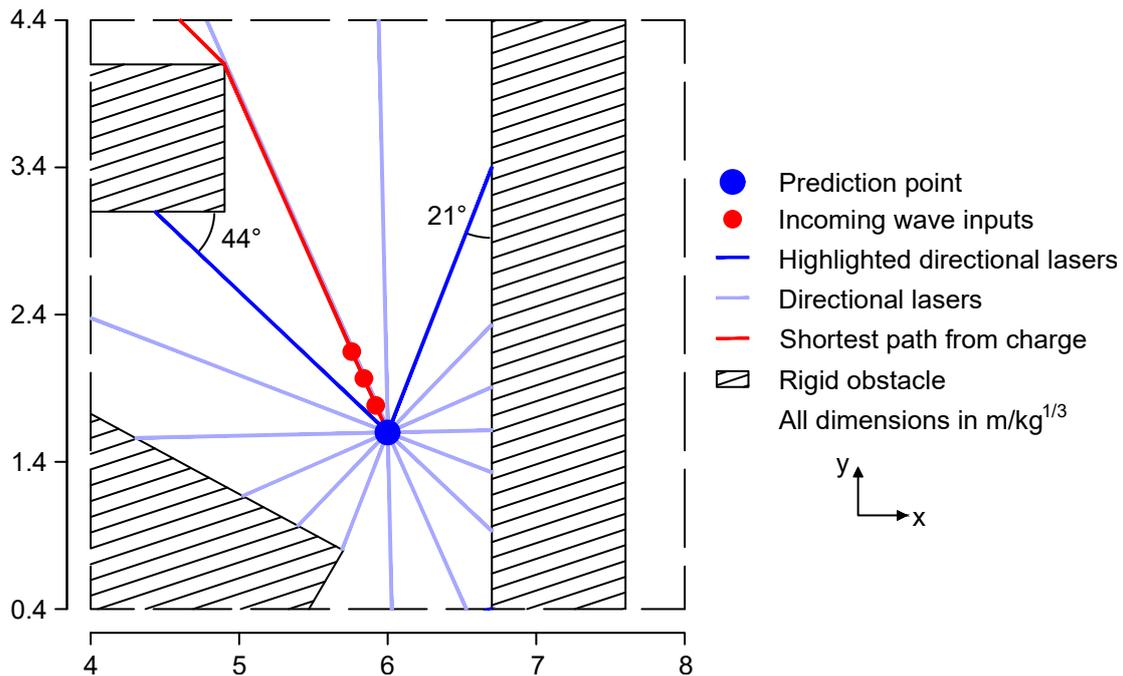
**Figure 3.** Example of the new input features allowing for predictions in more complex urban domains. Highlighted directional lasers correspond to angular inputs. Reduced domain and prediction point taken from Figure 1.
