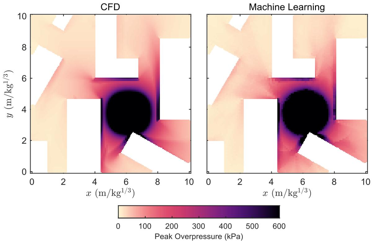
**Figure 6.** Comparison of the ML predictions and a CFD simulation of the same domain.
