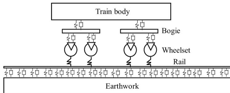
**Fig. 7** Vehicle-track-trackbed coupling calculation model
