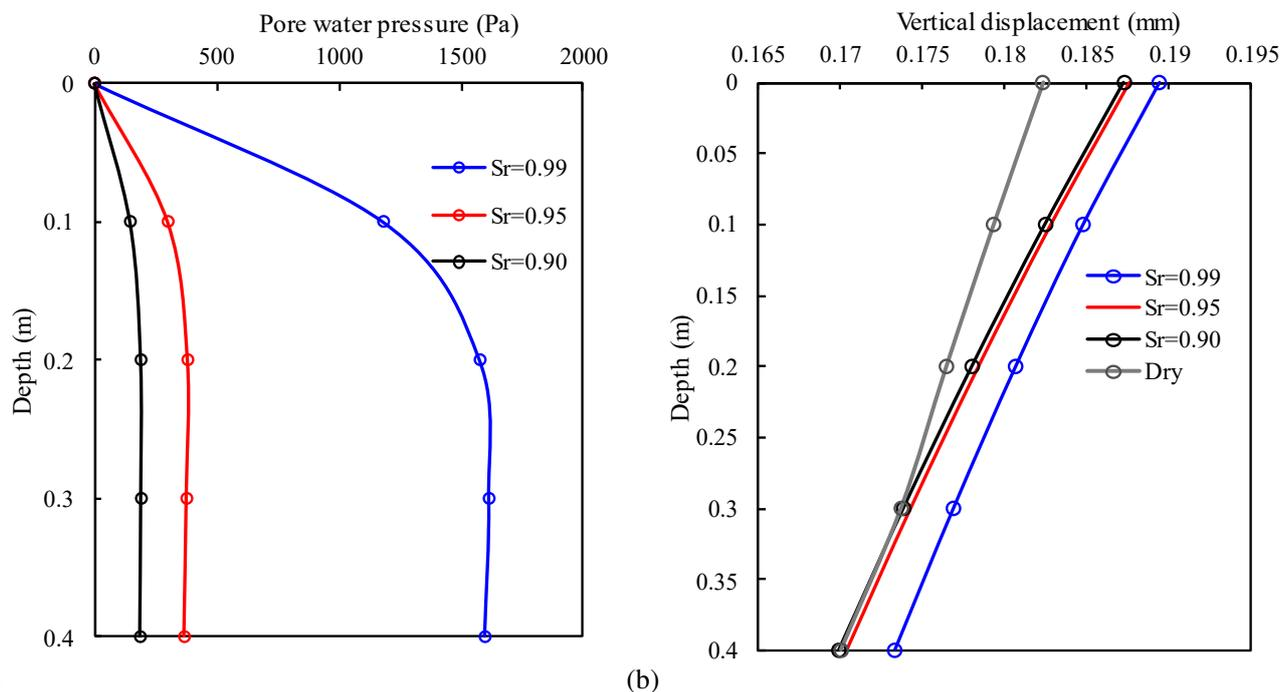
451 (a) 452 Fig. 14 The effect of the degree of saturation on the index of hydrodynamic response, (a) Pore water pressure, (b) Vertical
