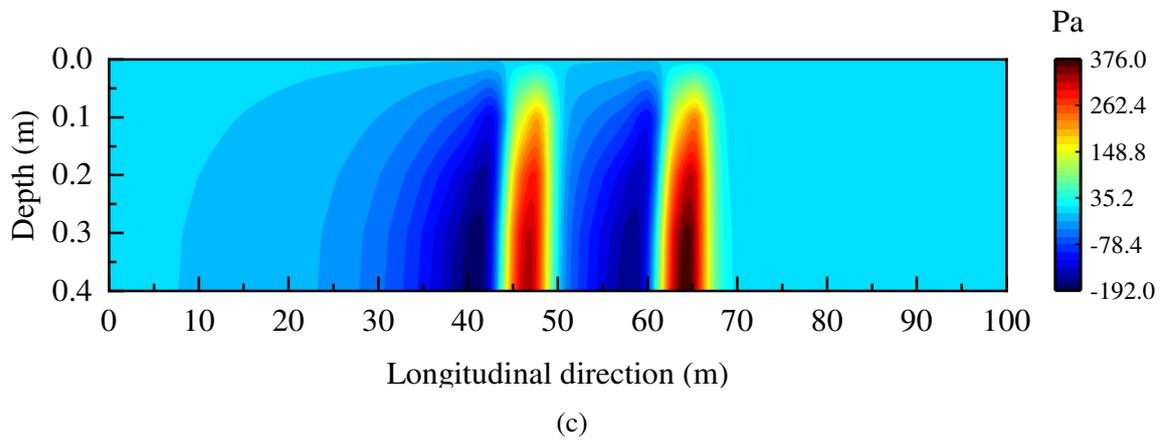
423 Fig. 13 Time-varying characteristics of dynamic response of unsaturated trackbed, (a) Pore water pressure, (b) Vertical
