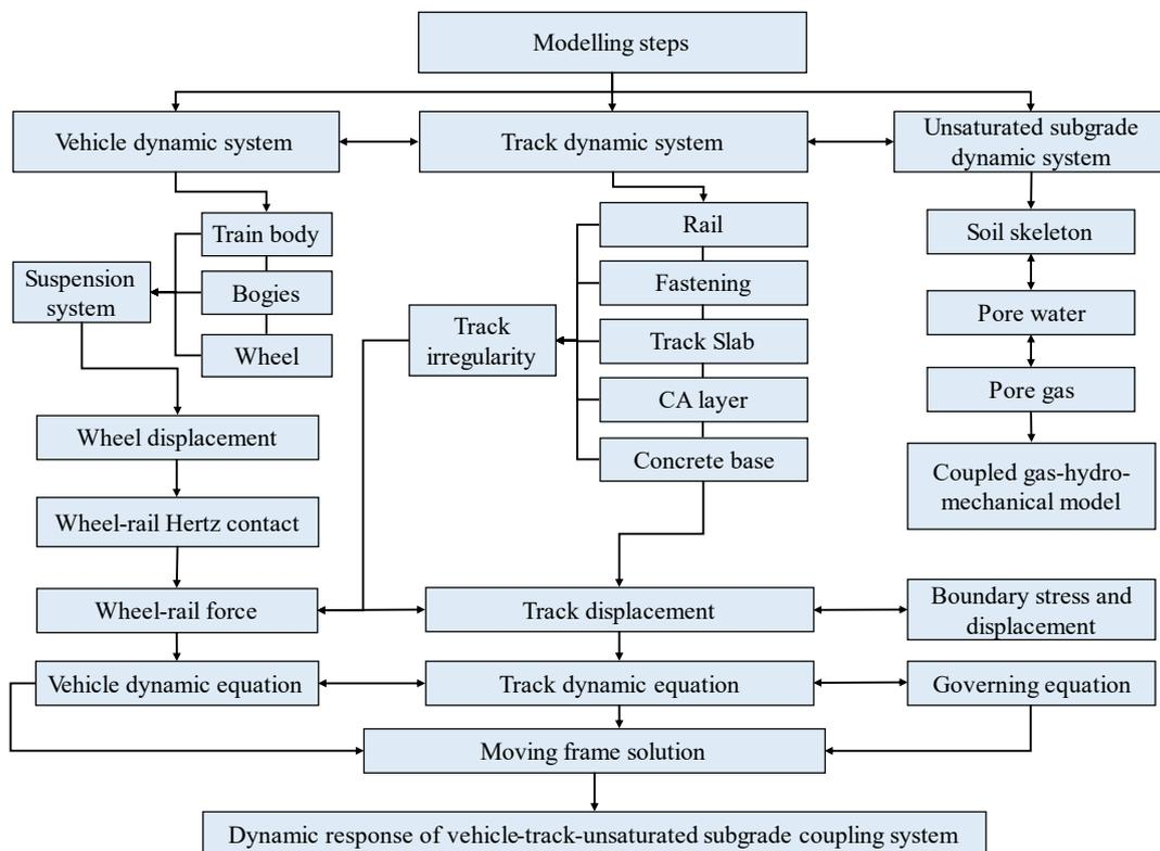
Fig. 2 Flowchart of the vehicle-track-unsaturated trackbed model
