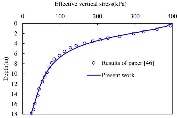
**Fig. 12** Comparison of calculation results of saturated foundation
