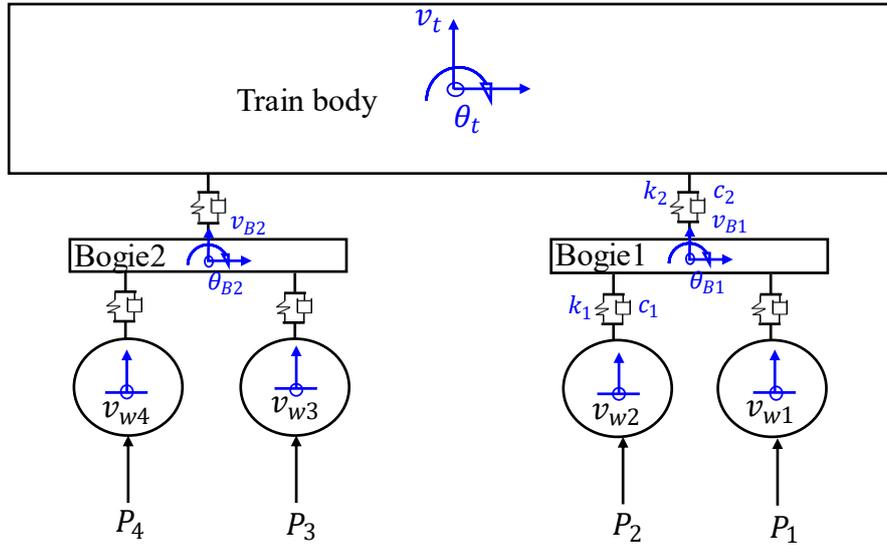
Fig. 4 Multibody vehicle model
