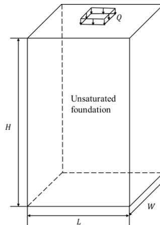
**Fig. 9** Calculation model of unsaturated foundation
