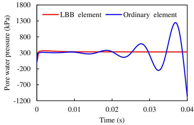
**Fig. 6** Comparison between the LBB stabilization method and the non-stabilization method
