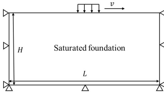
**Fig. 11** Calculation model of saturated foundation
