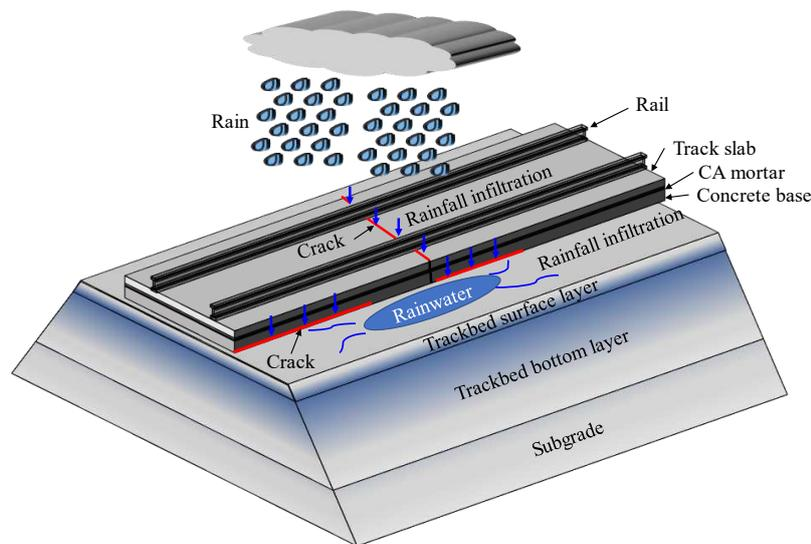
**Fig. 1** Infiltration of rainwater and evolution of water content within a ballastless trackbed
