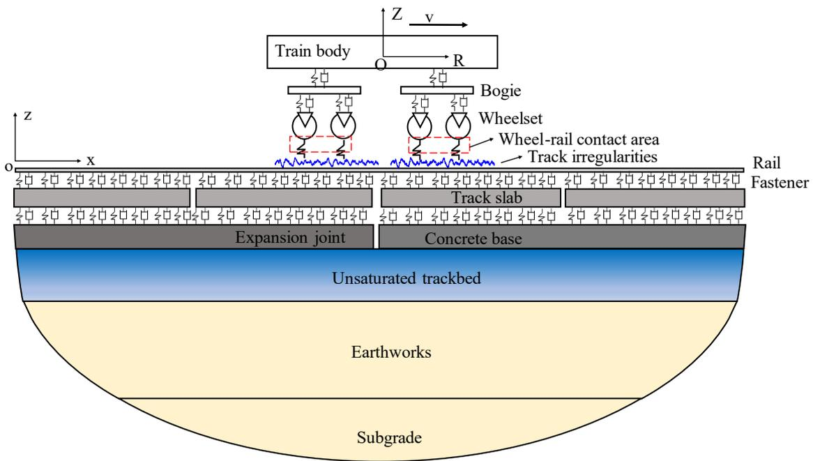
**Fig. 3** Mathematical modeling of the vehicle-track-unsaturated subgrade coupling system in a moving frame
