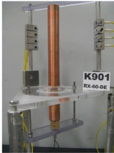
Figure 7. Set-up for confined tests of spherical plastic explosive charges
