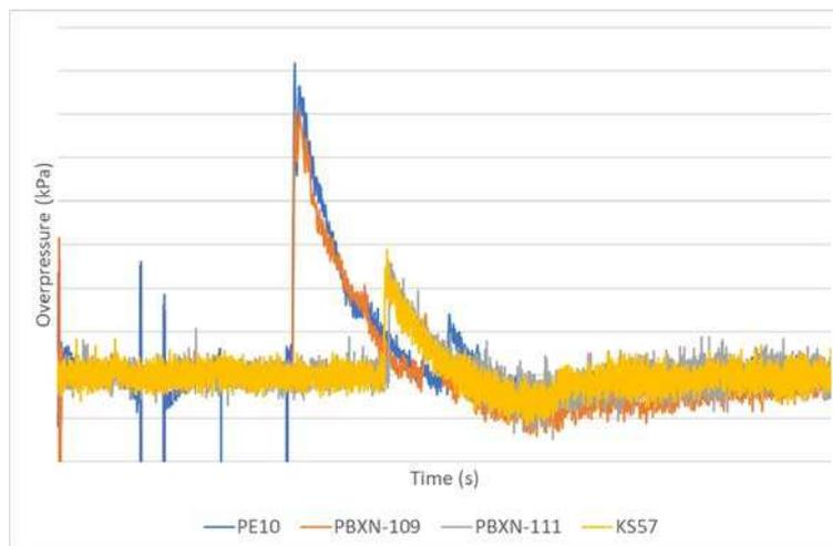
**Figure 7.** Comparison of test data for non-ideal explosives
