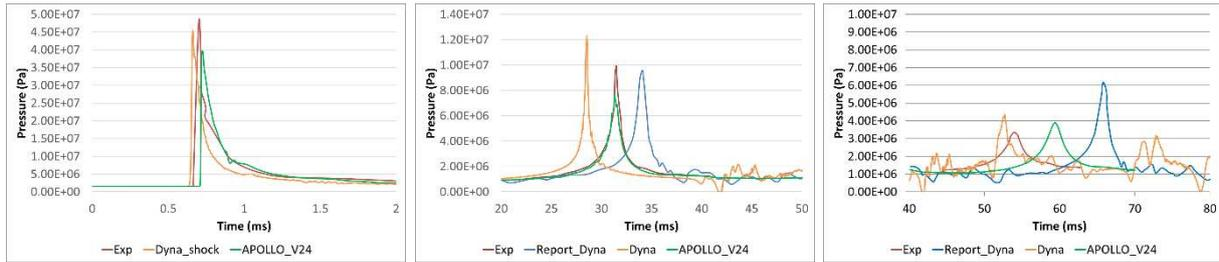
**Figure 2.** 1.13kg TNT sphere at a depth of 152.4m with a gauge distance of 1.26m; results displayed include test data, LS-DYNA and APOLLO
