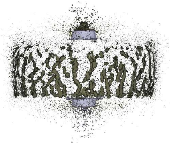
Figure 15. Natural fragmentation of a cased charge in IMPETUS
