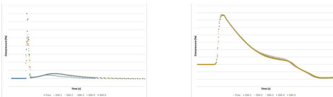
Figure 6. CompB porous functionality comparison against a standard JWL approach taken at a scaled distance of approximately 0.7 (left) and 11 \text{m/kg}^{1/3} (right)
