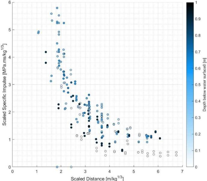
**Figure 8 – Scaled max specific impulse values against scaled distance with marker colour indicating the depth at which the pressure gauge is below the**
