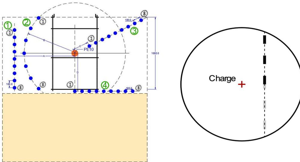
**Figure 1.** Schematic drawings showing mounting type 1 (left), the structural method with green numbering denoting the gauge position layouts, and mounting type 2 (right) which presents a plan view of the pressure gauges on thin cables affixed to tank walls.
