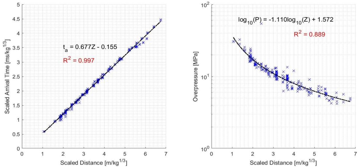
**Figure 6** - a) Scaled arrival time and b) peak overpressure against scaled distance for all underwater explosive trials whereby the charge was fully submerged in the water.
