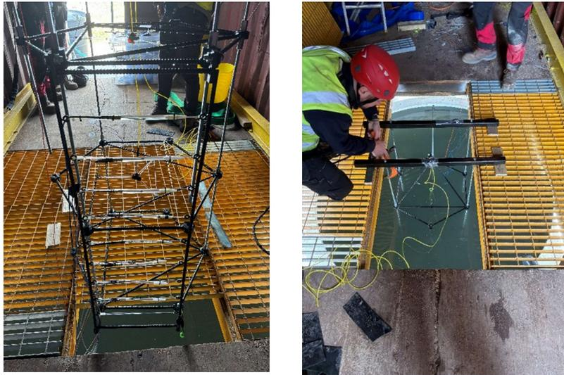
**Figure 2.** Photographs of the Mounting Type 1 – Structural Influencing with precise charge and gauge placement with respect to one another, showing both pre-test placement and in-situ of water.
