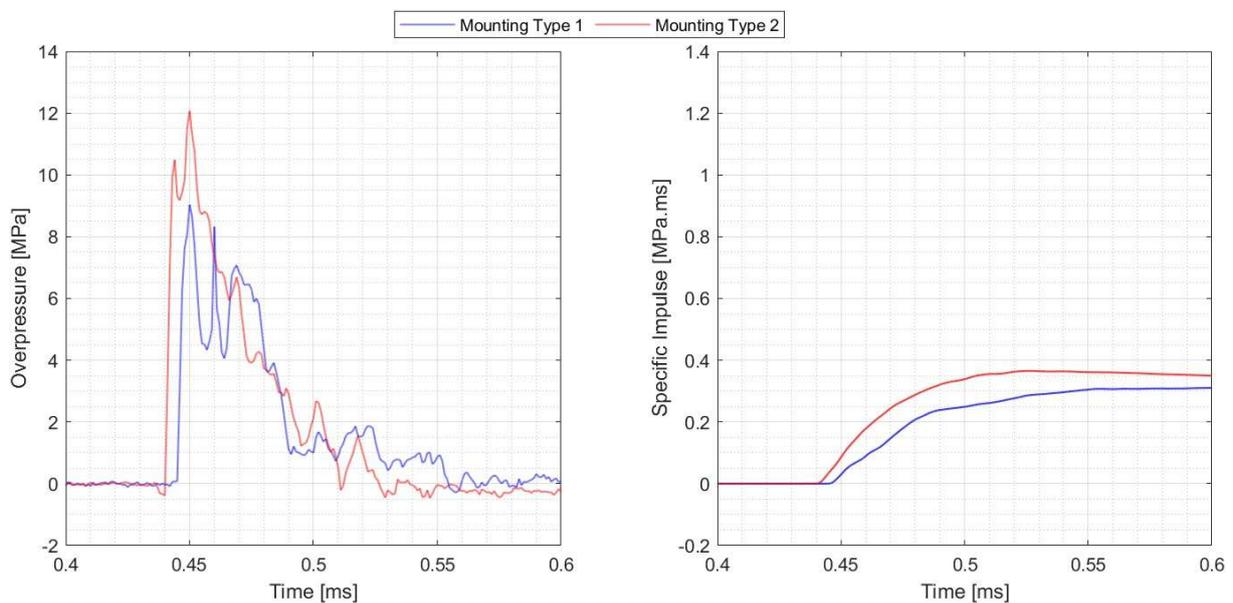
**Figure 4 – a) Pressure-time and b) specific impulse-time histories comparing the effects of mounting type on nominally identical test criteria**
