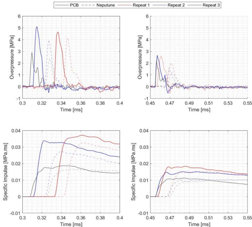
**Figure 9** – Comparative results between both gauge type measurements at 500mm (left) and 700mm (right) standoff distances, located at a 100mm depth, where the charge was floating on the water surface
