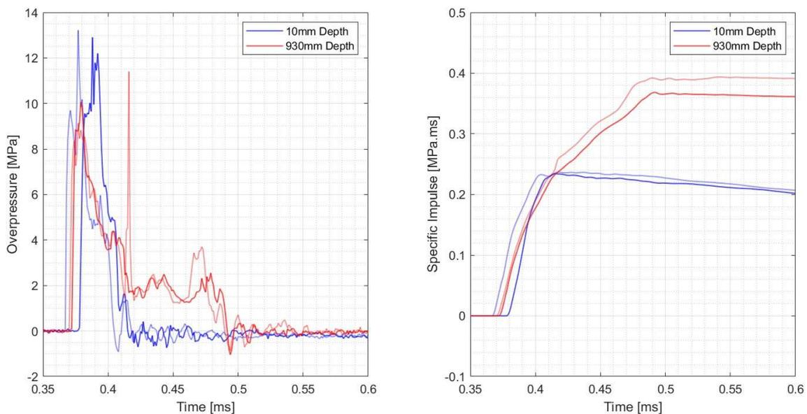
**Figure 7** - a) Pressure-time and b) specific impulse-time histories comparing the effects of gauge position regarding the proximity of the gauge to the water-air interface
