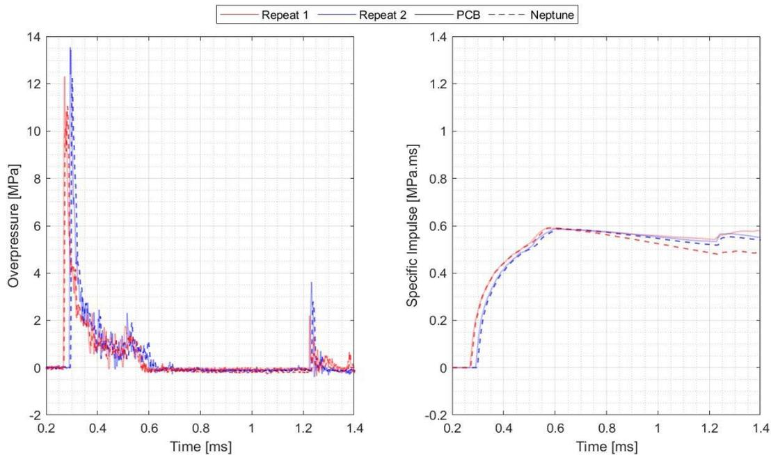
**Figure 5** - a) Pressure-time and b) specific impulse-time histories comparing the effects of gauge type on nominally identical test criteria
