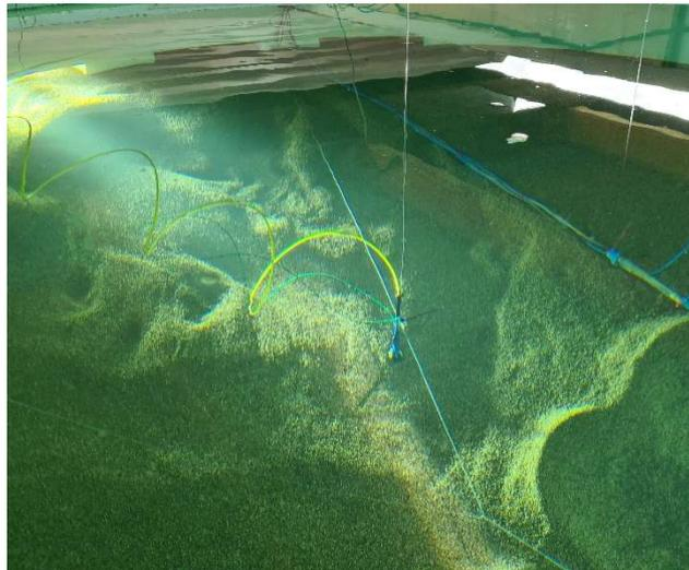
**Figure 3.** Photographs of the Mounting Type 2 – Minimal shock Influence with gauges and charge placed on thin wires but highly less control in placement
