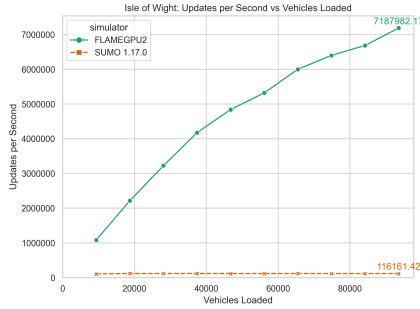
(c) Simulation state-change per second compared to the number of vehicles loaded.
