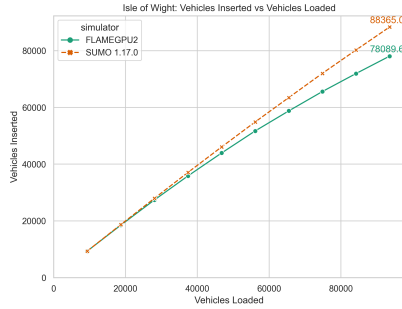
(d) Number of vehicles inserted into the model compared to the number of vehicles loaded.
