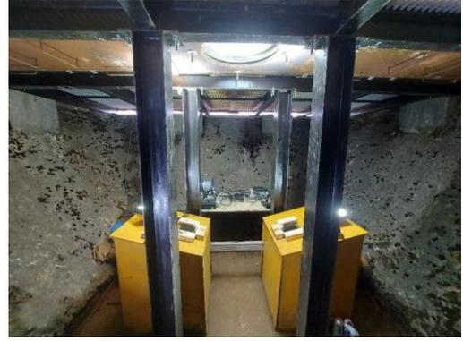
**Figure 3.** Experimental apparatus with soil container supported above HSV cameras
