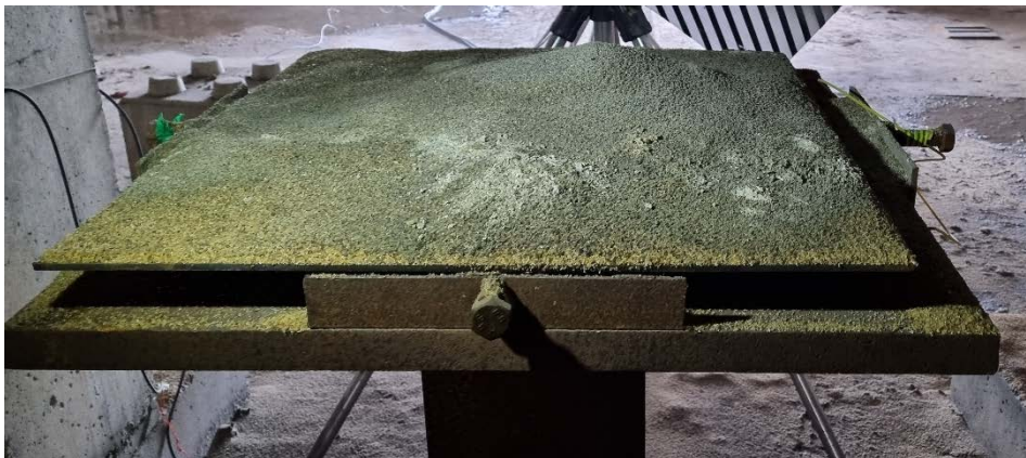
Figure 5. Post-test photos showing the sample is fully broken up during the blast over timescales much longer than of interest.
