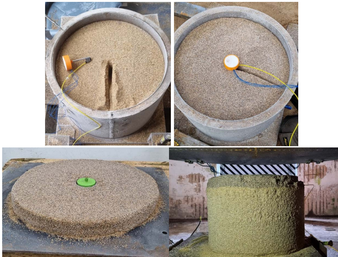
Figure 2. Images showing the different stages of burying a charge in a frozen soil bin. The top two show the channel dug out below the charge for the detonator and leads, the bottom left image shows the top ice slab with a former to create the void for the charge and the bottom right shows a frozen soil sample removed from the cardboard former prior to testing.
