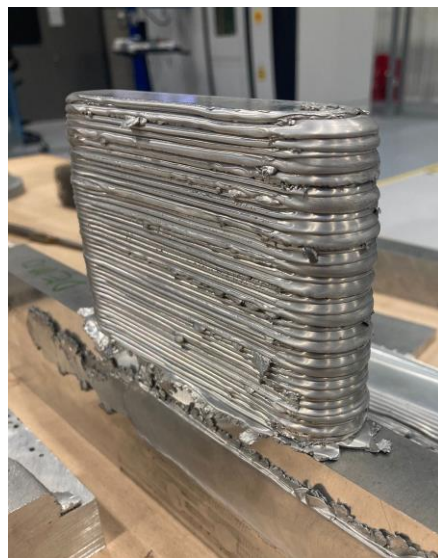
Figure 3. A single-track wall manufactured by AFSD in AA6xxx series.
