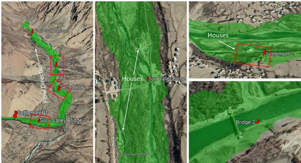
**Figure 13.** Buildings, roads, bridges and other infrastructure under potential threat of GLOF inundation in scenario (1) in the downstream flow channel of Panikhar lake.
