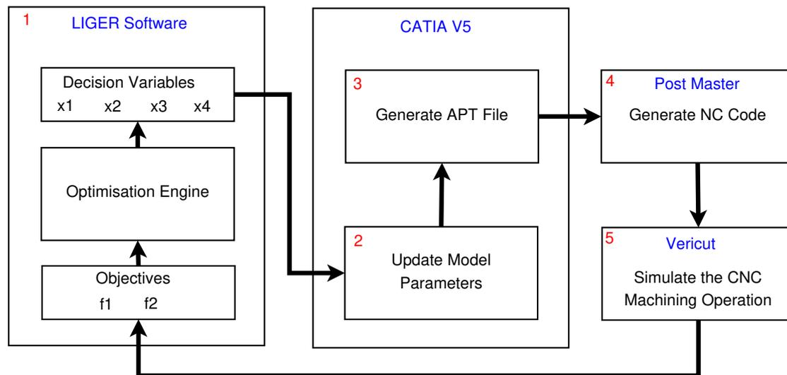
Fig. 2: Process flowchart for machining case study.
