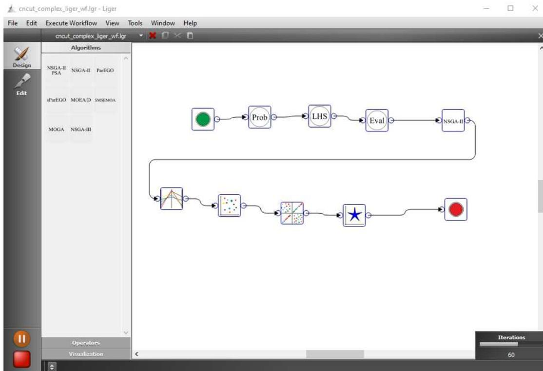
Fig. 1: Liger graphical user interface running an optimization workflow with the subtractive process planning problem.
