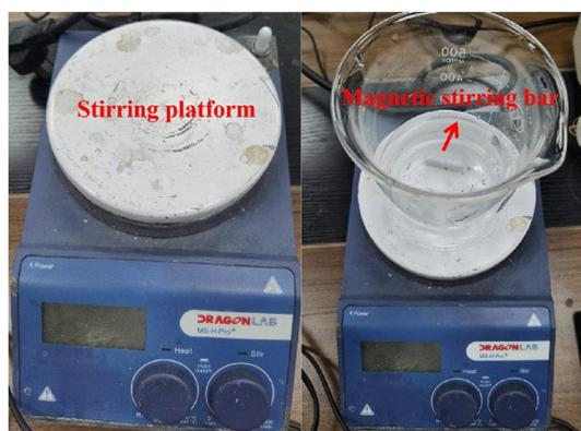
**Fig. 2.** Schematic of the magnetic stirrer. The left side shows the stirrer without a beaker, and the right side shows the stirrer with a beaker and a magnetic stirring bar placed inside. Once the stirrer is turned on, the magnetic stirring bar creates a stirring effect in the liquid.
