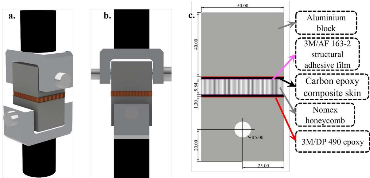
**Figure 3.** Schematic illustration of flatwise tensile test system: a. Isometric view, b. frontal view, and c. the configuration of the test components and the specimen adhered to the blocks.
