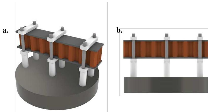
**Figure 5.** Schematic representation of the DMA specimen and testing in double cantilever mode: a. perspective view and b. front view.
