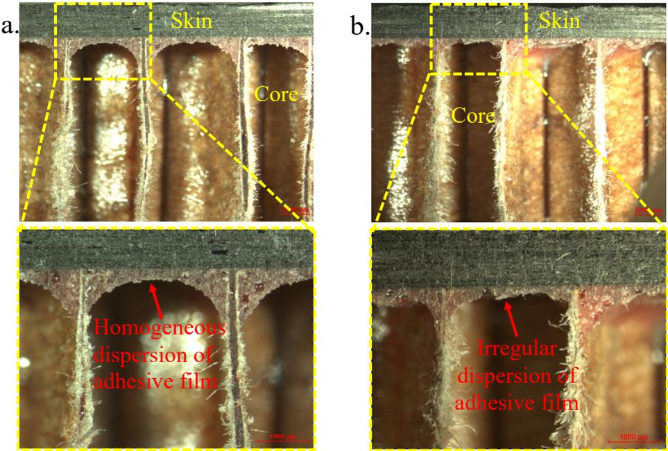
**Figure 7.** Microscopy images of cross-sections of a. APA-treated and b. NT specimens.
