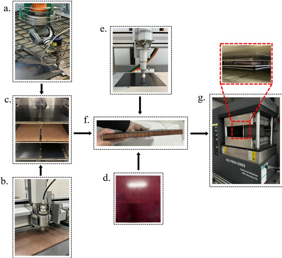
**Figure 2.** Composite sandwich manufacturing: a. Waterjet cutting of skin laminates, b. Digital cutting of honeycomb, c. Oven drying of skin and honeycomb cores, d. Preparation of 3M/AF 163-2 adhesive film, e. APA treatment of the composite specimens, f. Uncured
