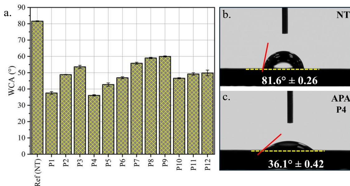
**Figure 6.** a. WCA values for NT and APA treated specimens; representative WCA images of b. NT and c. APA-treated surfaces.
