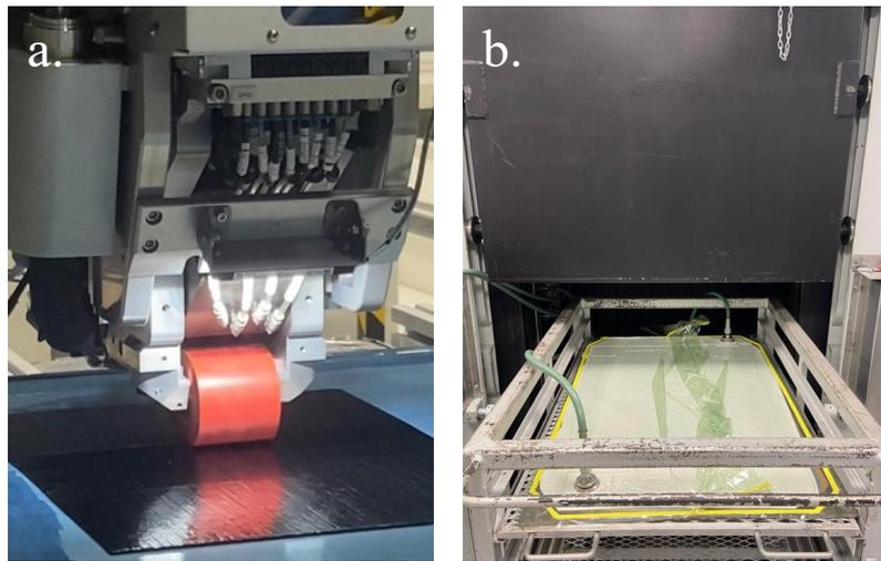
**Figure 1.** Composite skin manufacturing a. lay-up process with automated fiber placement and b. oven curing after 24 hours of debulking.
