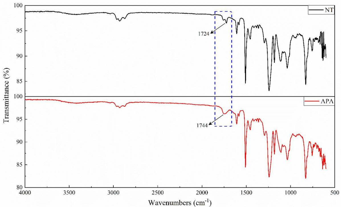
**Figure S1.** Fourier-transform infrared spectroscopy spectrums of before and after the atmospheric plasma activation (APA) of composite skins.
