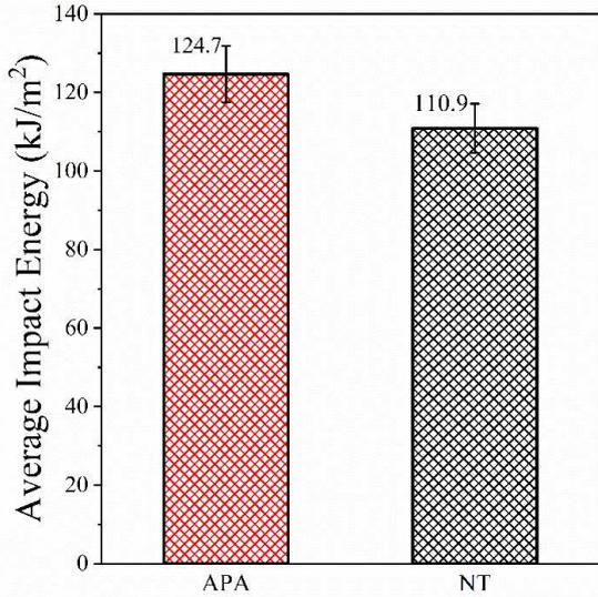
**Figure 10.** Average impact energy (kJ/m<sup>2</sup>) values of APA-treated and NT specimens.
