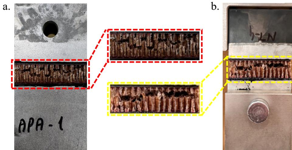
**Figure 9.** The fractured region of Nomex honeycomb core after flatwise tensile tests:
