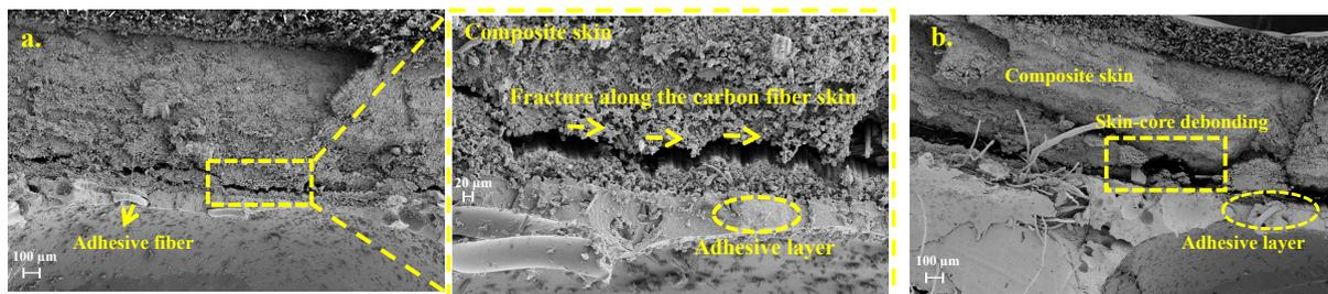
**Figure 11.** Scanning Electron Microscope (SEM) images for a. APA-treated and b. NT specimens.
