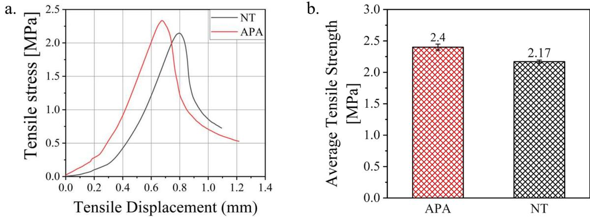
**Figure 8.** a. Tensile stress-displacement curves of APA-treated and NT sandwich composite specimens and b. Average tensile strength values of APA-treated and NT sandwich composite specimens.
