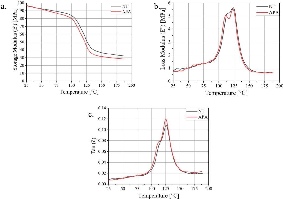
**Figure 12.** DMA curves of APA -treated and NT specimens for a. Storage Modulus ( $E'$ ), b. Loss Modulus ( $E''$ ) and c.  $\tan(\delta)$ .
