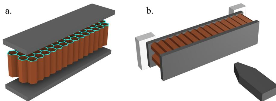
**Figure 4.** Schematic representation of Charpy impact test: a. components of the sandwich specimen and b. testing configuration.
