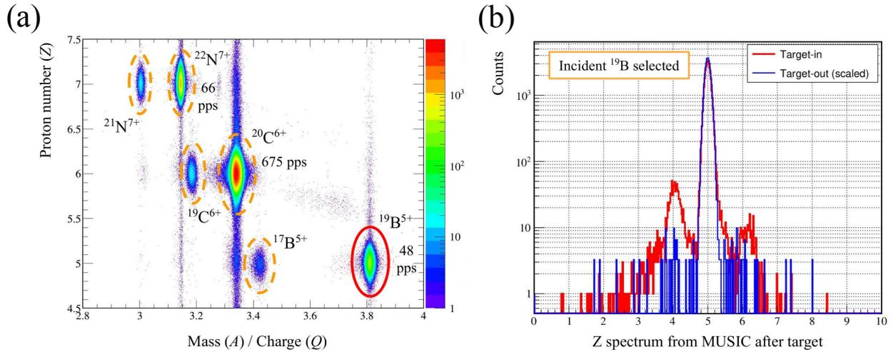
Figure 3: (a) Particle identification with ZDS detectors before the reaction target. Nuclear species and their rate are indicated (b) Z spectrum of the MUSIC after the reaction target for with (red) and without (blue) target conditions.
