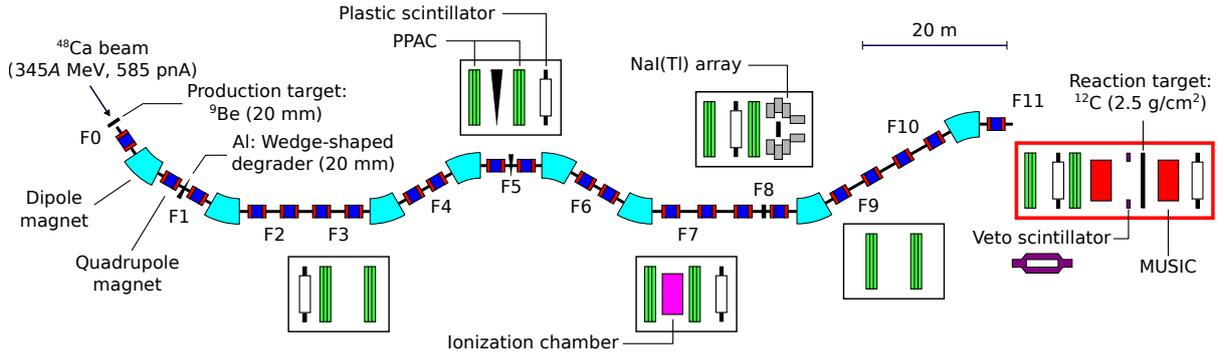
Figure 2: BigRIPS (F0 to F7) and ZDS spectrometer (F8 to F11) schematic showing detector arrangement for  $\sigma_{cc}$  measurement of  $^{19}\text{B}$  at the F11 focal plane.
