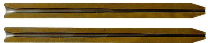
Fig. 4. Worn mixing tubes 1 (top) and 2 (bottom) after longitudinal sectioning using electrical discharge machining (EDM). The EDM wire was offset to get one perfect half that is displayed above.
