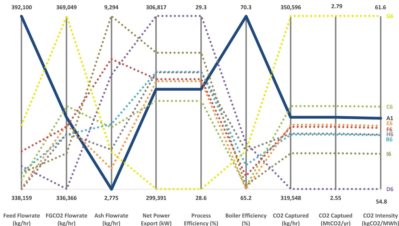
Fig. 13. Parallel plot for BECCS KPI comparison between each case study.
