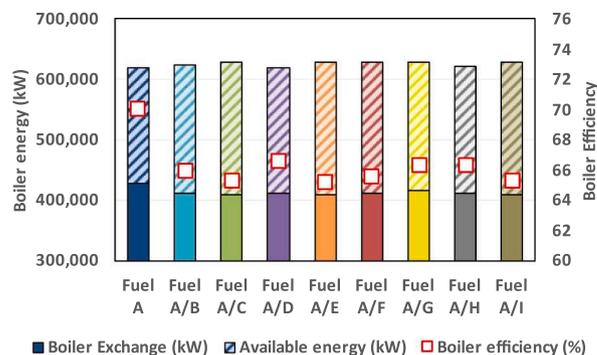
**Fig. 12.** Boiler efficiency and amount of available heat remaining in the boiler for the 70:30 fuels blends.
