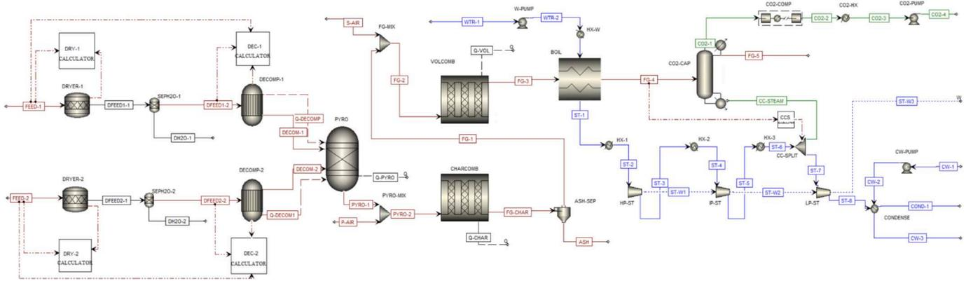
Fig. 3. Baseline BECCS power plant model topology developed in Aspen Plus. Biomass combustion, power generation, and CO<sub>2</sub> capture are shown in red, blue, and green, respectively.
