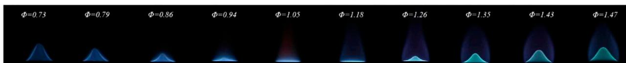
**Figure 2.** Methane flames with  $\Phi$  ranging from 0.73 to 1.4.
