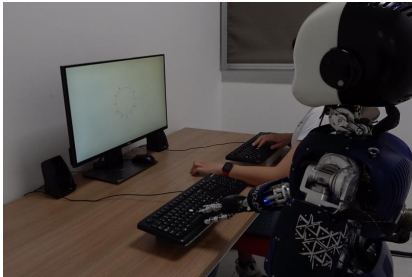
Fig. 2. An example experimental paradigm for studying SoA in a human-robot interaction. The photograph illustrates a joint action paradigm where the two partners (here a human participant and the iCub humanoid robot) are responsible for complementary actions [134]. The task is to judge the occurrence (the moment in time) of an auditory beep produced by a keypress of one of the partners. If SoJA is formed, then participants should show temporal compression (temporal binding) between the keypress and the auditory tone, regardless of who actually produced the keypress (themselves or the partner). In [134], participants formed SoJA with the robot when they attributed intentional agency to it.
