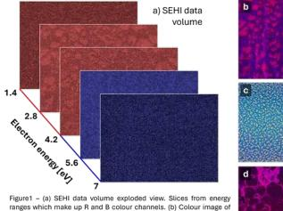
Figure1 – (a) SEHI data volume exploded view. Slices from energy ranges which make up R and B colour channels. (b) Colour image of lithium metal formed from summed colour channels as shown in (a). (c) Spider dragline silk, (d) Organic-inorganic lead iodide solar cell material. Figures and data adapted under CC BY 4.0 licence from [1].
