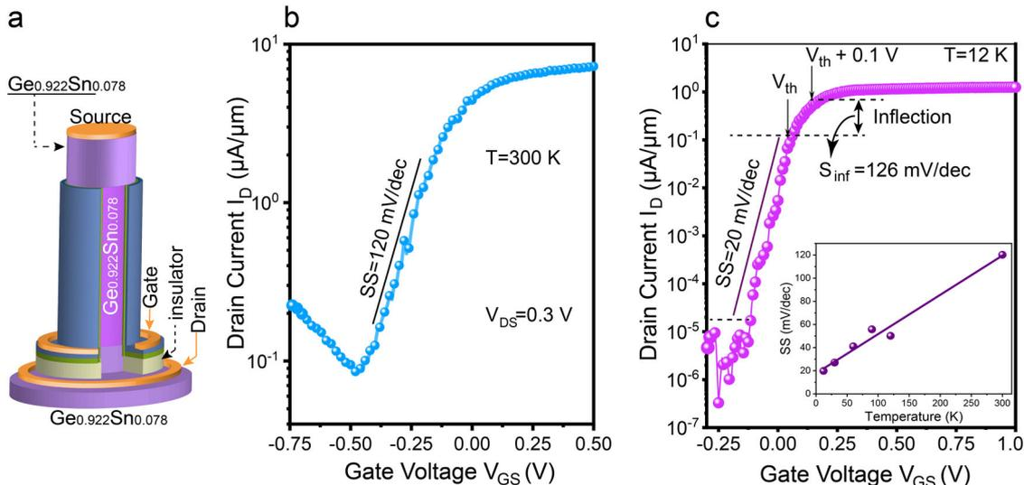
**Fig. 6 Characteristics of an all  $\text{Ge}_{0.922}\text{Sn}_{0.078}$  vertical n-FET (n-VFET) with a nanowire (NW) diameter of 50 nm.** **a** Schematic showing the device structure; **b**  $I_D$ - $V_{GS}$  transfer characteristics measured at 300 K and, **c** at 12 K. The inset in **c** shows the SS scaling with temperature. The steep slope in the inflection region demonstrates high potential for quantum computing application.
