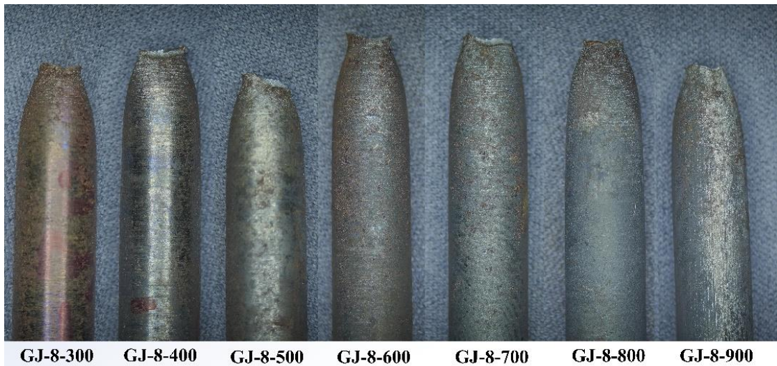
Fig. 9. Typical fracture site side view photos of specimens after testing.
