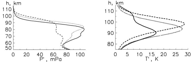
Figure 2: Change in pressure  $p'$  (a) and temperature  $T'$  (b) with the altitude as a result of passing of an AGW with a period of 65 minutes and  $k_x = 10^{-5} \text{ m}^{-1}$  (solid line - 18 July 2005, dashed line - 28 August 2005, dotted line - 19 October 2005).
