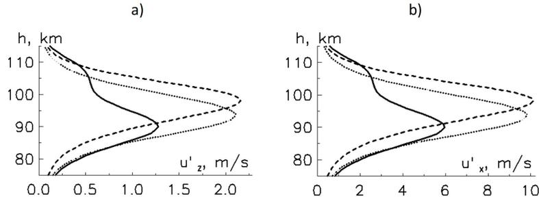
Figure 1: Change in vertical  $u'_z$  (a) and horizontal  $u'_x$  (b) component of velocity with altitude, as a result of passing of an AGW with a period of 65 minutes and  $k_x = 10^{-5} \text{ m}^{-1}$  (solid line - 18 July 2005, dashed line - 28 August 2005, dotted line - 19 October 2005).
