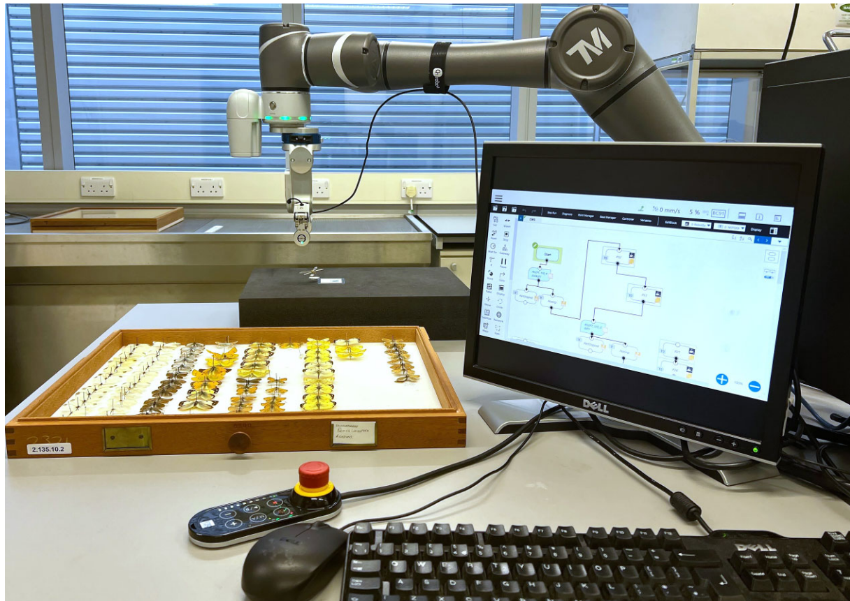
Fig. 6 A Techman 500 robotic arm in action at the Natural History Museum, London, placing down a sample pinned specimen from a Lepidoptera collection. Here, the robotic arm has been trained to locate the specimen from the drawer, and then pick it up and place it on a board in order to scan the specimen. Synthetic specimens were used in the training stage for this task.
