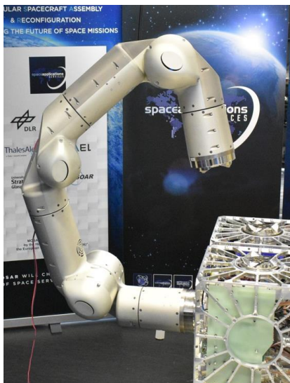
Figure 7: Relocatable robotic arm for in-orbit servicing.
