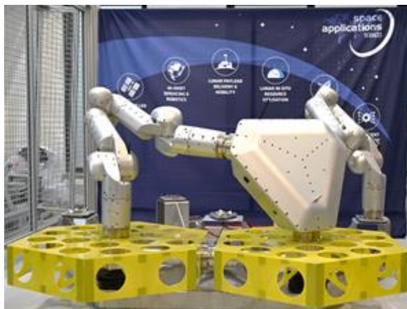
Figure 8: Multi-arm modular robot for large telescope assembly.
