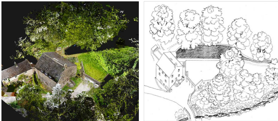
Figure 15. The juxtaposition of the building-in-site axonometric post-produced after scanning (left) (Image by authors); The original design drawing (right) (Image by Peter Blundell Jones)
