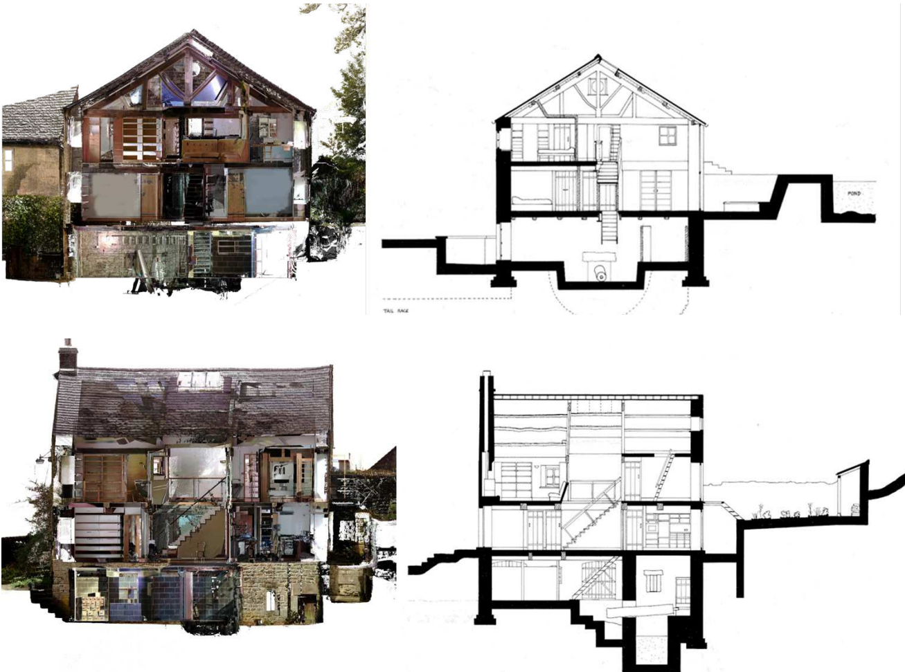
Figure 18. The juxtaposition of the longitudinal section post-produced after scanning (left) (Image by authors); The original design section (right) (Image by Peter Blundell Jones)
