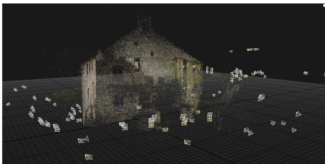
Figure 7. Various camera points from the exterior of the building which were used for photogrammetry (Image by authors)
