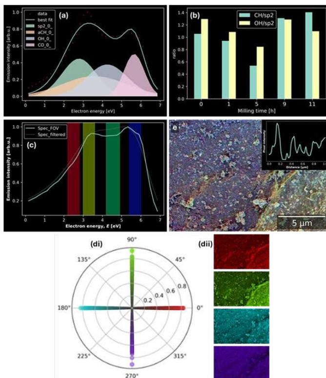
Figure 1 – (a) Component fit to average SE spectra for material produced by 5h ball milling. (b) CH: $sp^2$  and OH: $sp^2$  ratio plots for each ball milling time. (c) energy ranges assigned to spaced colour hue channels (fi) to make component images (fii) summed to make the colour image in (e). (e – inset) line profile showing nanoscale satellite particle morphologies.
