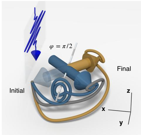
**Fig. 2 | Diagram of example magnetisation vector during switching.** Sublattice magnetisation vectors switching from  $\langle 110 \rangle$  to  $\langle -110 \rangle$  with  $\epsilon \parallel \langle 010 \rangle$ . (Opaque): initial orientation. (Bar): precession axis. (grey):  $t_p = 400$  fs,  $I = 2$  GW/cm<sup>2</sup>, (gold):  $t_p = 400$  fs,  $I = 4$  GW/cm<sup>2</sup>, and (blue):  $t_p = 3$  ps,  $I = 5$  GW/cm<sup>2</sup> ( $z$  magnetisation scaled 100× for visibility).
