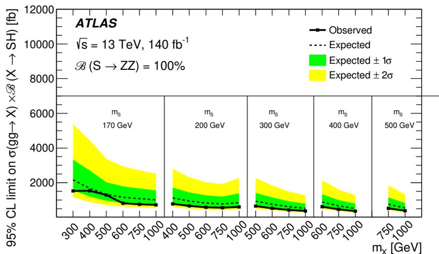
**Figure 8.** Observed (solid line) and expected (dashed line) 95% CL upper limits on  $\sigma(gg \rightarrow X) \times \mathcal{B}(X \rightarrow SH)$  as a function of  $m_X$  and  $m_S$ , under the assumption of  $\mathcal{B}(S \rightarrow ZZ) = 100\%$ . The green and yellow shaded areas indicate the  $\pm 1$  and  $\pm 2$  standard deviations around the expected limit.
