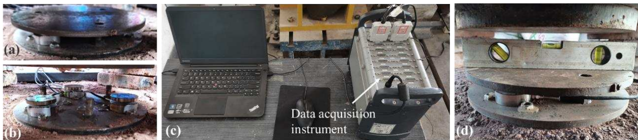
581 582 Fig. 18. Force measurement system: (a) force-measuring device; (b) load cell configuration; (c) microcomputer and 583 data acquisition instrument; (d) site levelling.
