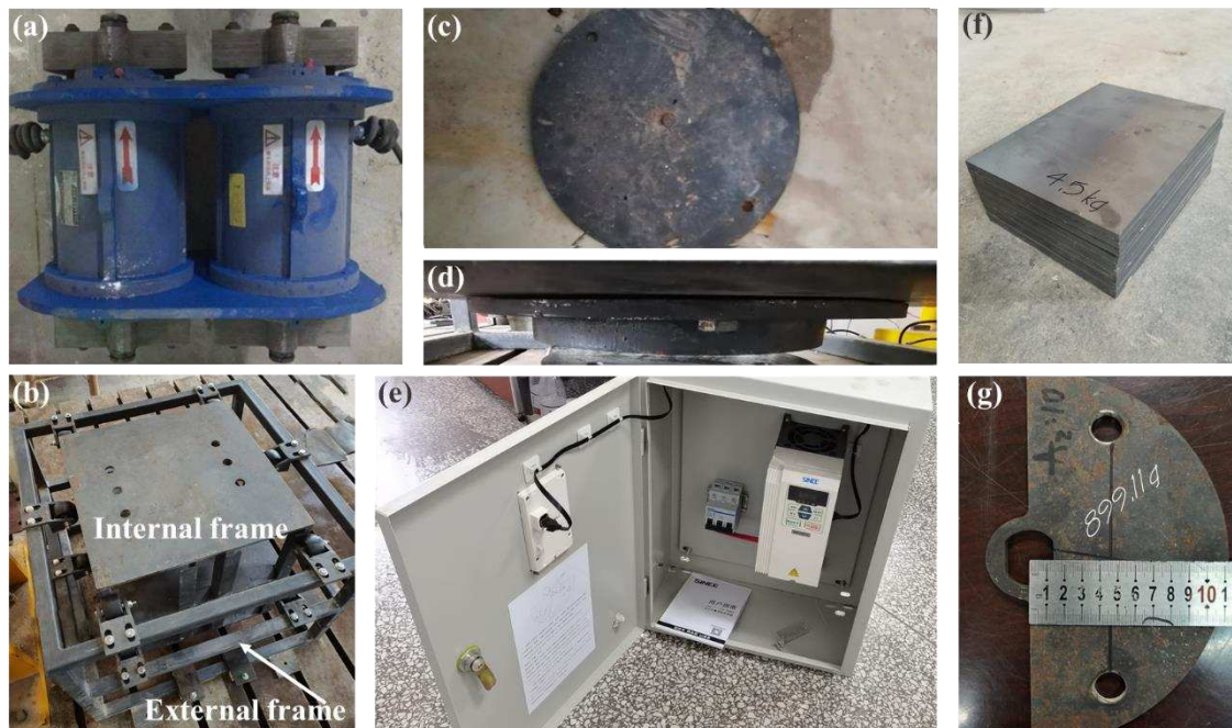
553 554 Fig. 16. Shaker components: (a) motors; (b) internal and external frame; (c) top view of the loading plate; (d) side 555 view of loading plate; (e) frequency modulator; (f) counterweight blocks; (g) eccentric block.
