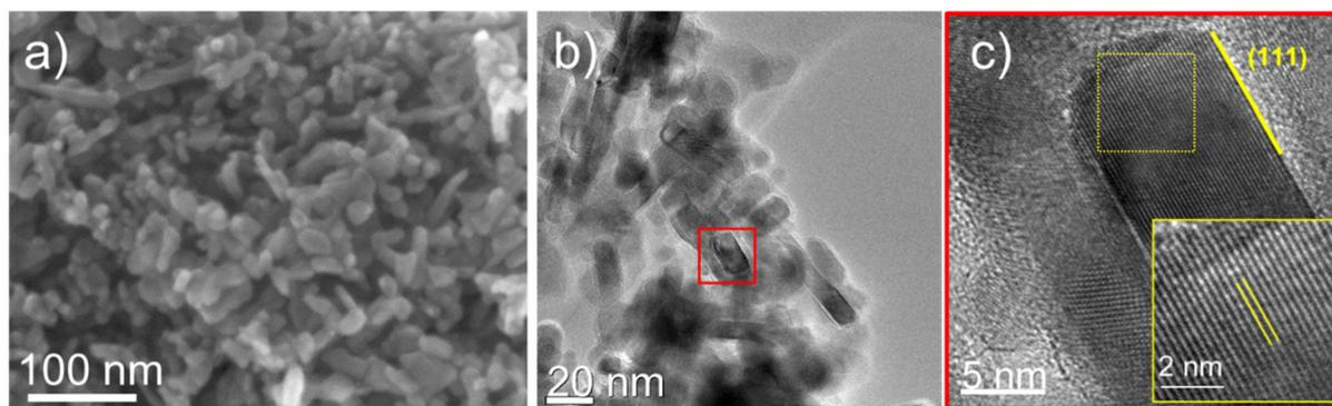
Fig. 7 (a) SEM image of NiO NPs obtained with thermal treatment of  $\text{Ni}_3(\text{OH})_4(\text{NO}_3)_2$ , (b) TEM image of NiO NPs, and (c) HRTEM images of selected NiO NPs, outlined in (b) with the red square. The inset in (c) shows the {111} atomic planes of NiO.
