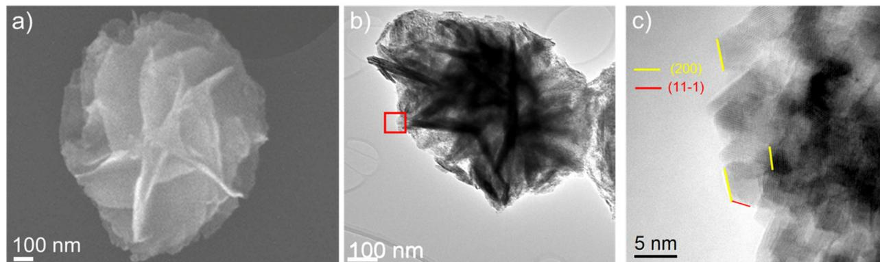
**Fig. 6** (a) SEM image of NiO obtained with thermal treatment of  $\beta$ -Ni(OH)<sub>2</sub> flower-like nanostructure, (b) TEM image of annealed NiO nanoflower particle, and (c) HRTEM images of the red marked region in (b) outlining the NiO NPs with (111) atomic planes of NiO from a single particle shown in the inset.
