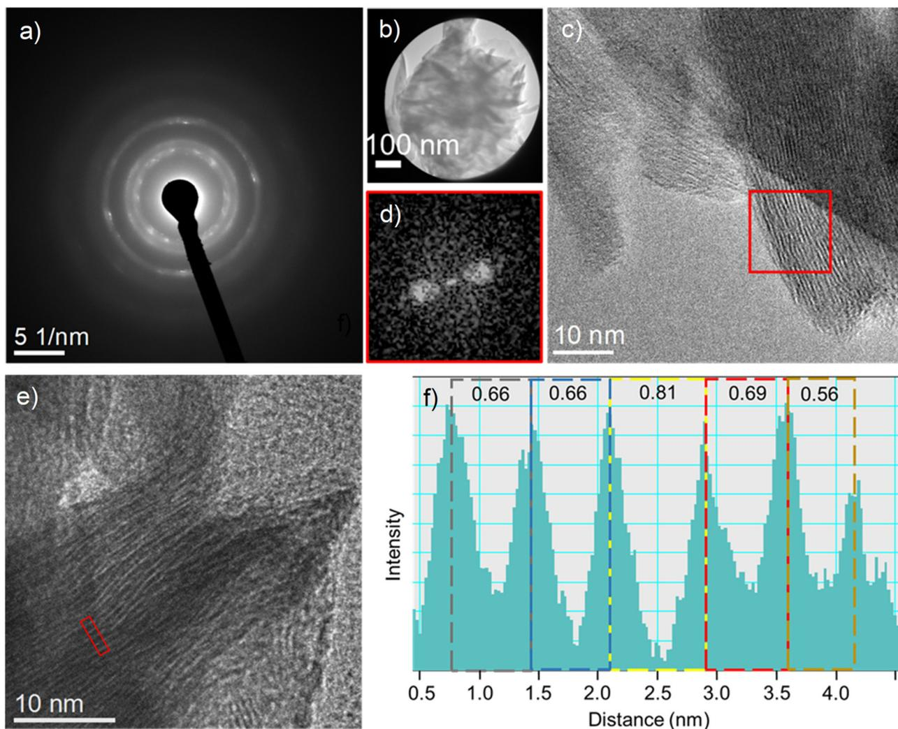
**Fig. 4** (a) Electron diffraction of a single flower-like nanostructure (b), diffraction rings corresponding to  $\text{Ni}_3(\text{OH})_4(\text{NO}_3)_2$ , (c) an HRTEM image of  $\text{Ni}_3(\text{OH})_4(\text{NO}_3)_2$  nanoplates with digital diffractogram from highlighted regions shown in (d) showing the variation in atomic spacing planes highlighted by the real space intensity profile of (003) atomic spacing (f) taken from a region of HRTEM image of the nanoplate in (e).
