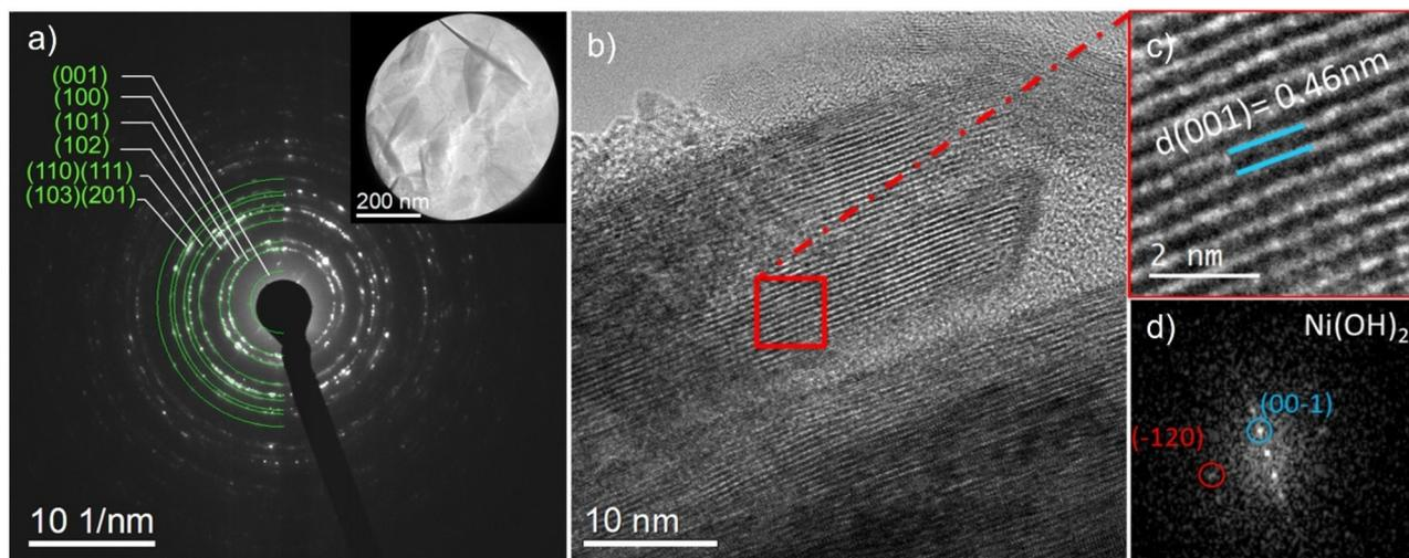
**Fig. 3** Electron diffraction of a single flower-like nanostructure (a) with diffraction rings corresponding to  $\beta$ -Ni(OH)<sub>2</sub> (the inset shows that they are from where diffraction was taken). (b and c) HRTEM images of  $\beta$ -Ni(OH)<sub>2</sub> nanoplates with (001) planes outlined, and (d) a digital diffractogram from (b), outlining (001) plane 'reflections'.
