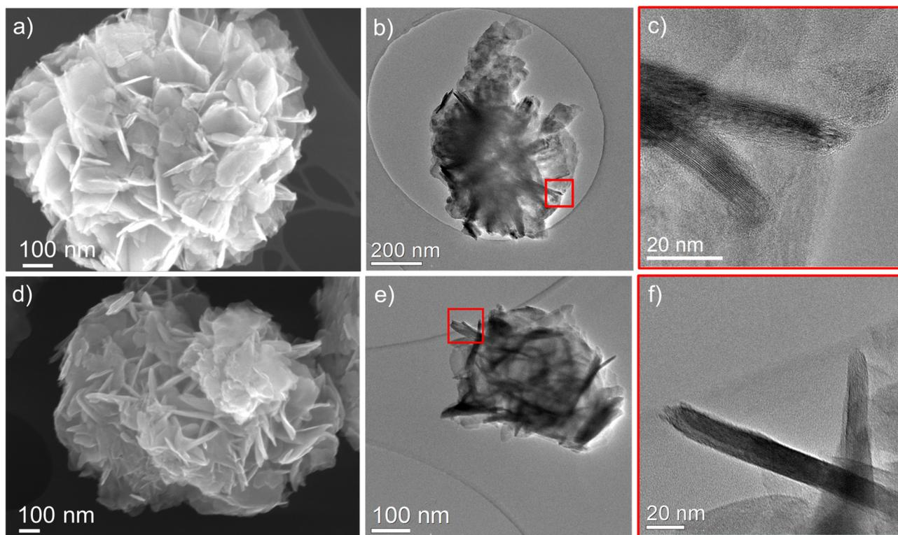
**Fig. 2** SEM and TEM images of the intermediates. Flower-like self-assembly of (a)  $\beta$ -Ni(OH)<sub>2</sub> and (d) Ni<sub>3</sub>(OH)<sub>4</sub>(NO<sub>3</sub>)<sub>2</sub> obtained through SEM, and TEM images of  $\beta$ -Ni(OH)<sub>2</sub> (b and c) and Ni<sub>3</sub>(OH)<sub>4</sub>(NO<sub>3</sub>)<sub>2</sub> (e and f) at different magnifications, showing their overall morphology and single nanoplates.
