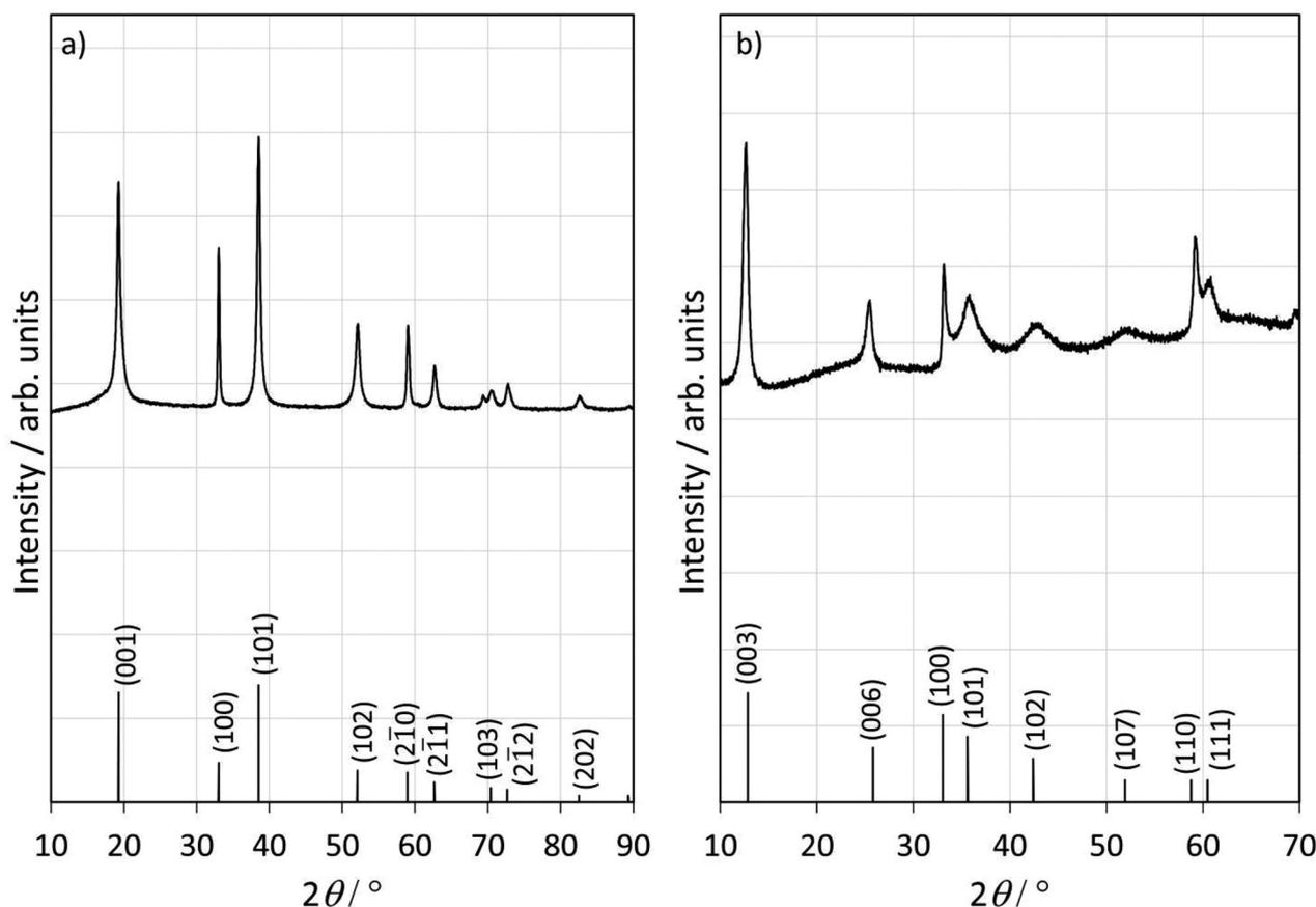
**Fig. 1** XRD patterns of intermediates in the case of ammonia (a) and carbamide (b) as hydroxide precursors and the corresponding bulk reference XRD of  $\beta$ -Ni(OH)<sub>2</sub> and Ni<sub>3</sub>(OH)<sub>4</sub>(NO<sub>3</sub>)<sub>2</sub>. Reference diffraction peaks are taken from ref. 66 and 67.
