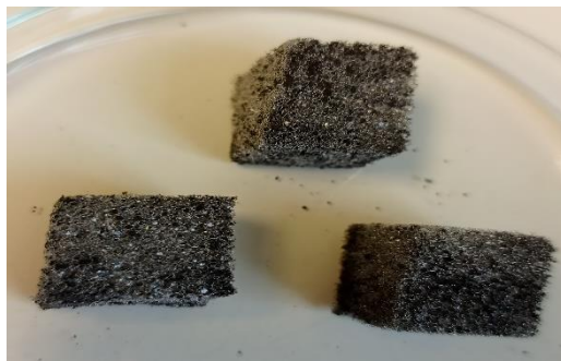
Fig. 1: Photo of polyurethane sponges coated with graphitic materials.
