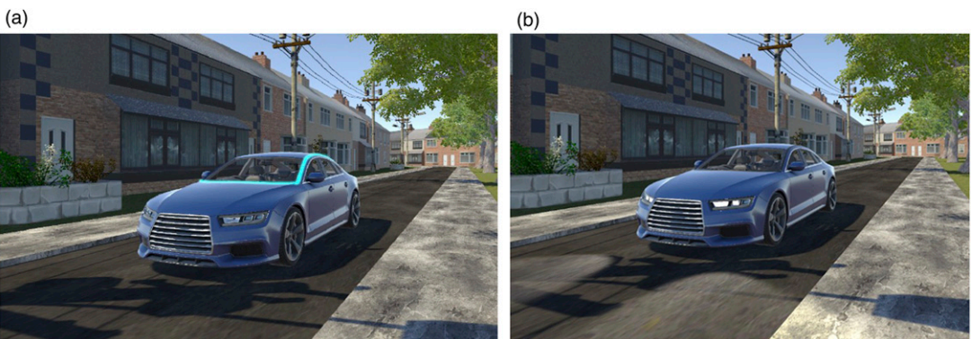
Figure 4. eHMI designs. (a) Slow Pulsing Light Band; (b) Flashing Headlights: Note the illumination on the road.
