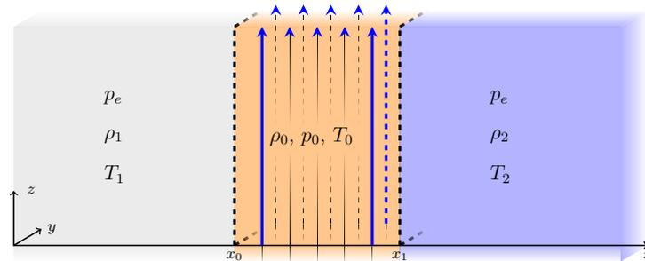
**Figure 3.** The model of a magnetic slab in an asymmetric non-magnetic environment (based on Figure 1 of Allcock and Erdélyi [84]). To keep the external pressures balanced, in accordance with Equation (3), they take the same value ( $p_1 = p_2 = p_e$ ), although the corresponding combinations of density and temperature may be different.
