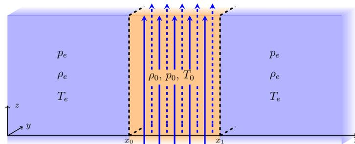
**Figure 2.** The model of a symmetric slab in a non-magnetic environment (figure based on Roberts [48]). Here, and in all the asymmetric slab systems that follow, stratification occurs in the  $x$ -direction only, while the system is generally infinite in the other two directions.
