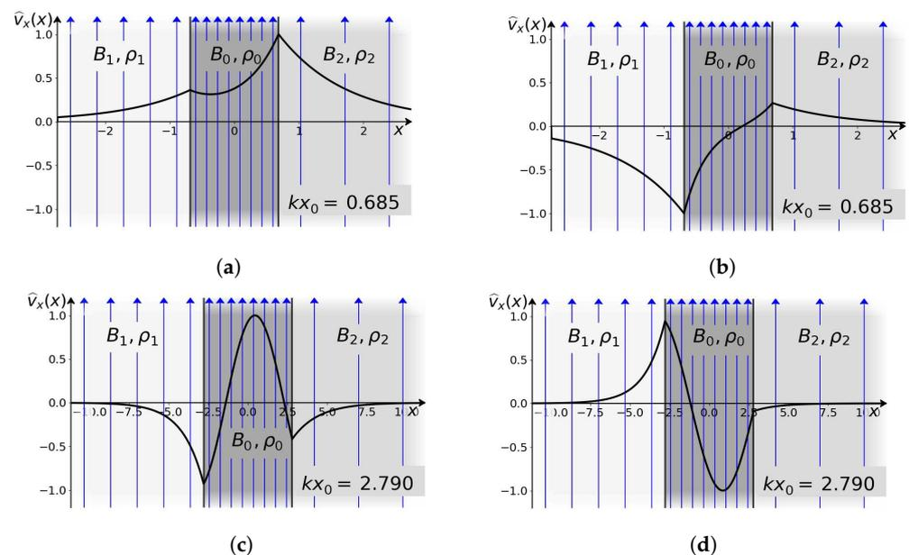
**Figure 4.** The transverse velocity perturbation amplitude of eigenmodes in an asymmetric magnetic slab, adapted from Figure 4 of Allcock et al. [46]. Panels (a,b) show a quasi-kink- and a quasi-sausage surface mode, respectively, in a thin slab. Panels (c,d) depict a quasi-kink and a quasi-sausage body mode in a wider slab. In all four cases, the slab is strongly magnetised and embedded in a rarefied asymmetric environment.
