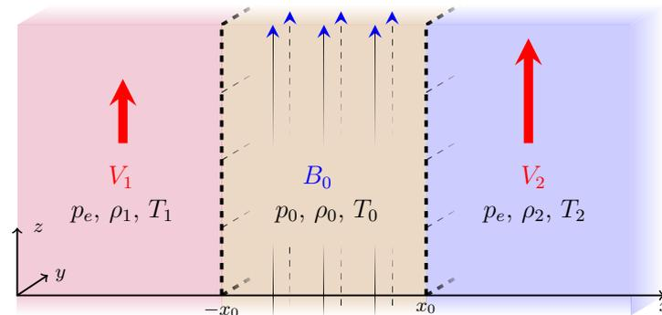
**Figure 8.** The model of a magnetic slab surrounded by different flows in its asymmetric non-magnetic plasma environment (based on Figure 1 of Zsámberger et al. [98]). Similar to the case illustrated in Figure 3, the external pressures are the same, while the other parameters are allowed to break symmetry.
