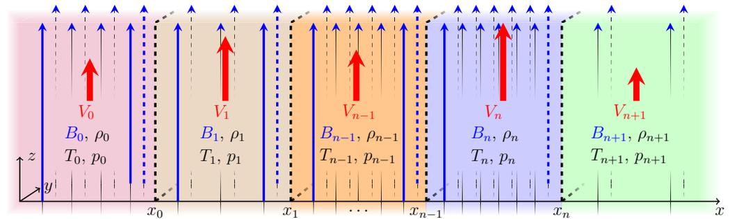
**Figure 1.** Generalised multi-layered Cartesian waveguide model including asymmetric flows. Structuring is present in the  $x$ -direction, while the system is infinite and non-stratified in the  $y$ - and  $z$ -directions.
