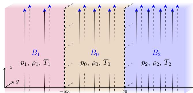
**Figure 5.** The model of a magnetic slab in an asymmetric magnetic environment, where both the plasma parameters and the magnetic field strength may take different values in the two external regions (adapted from Figure 1 of Zsámberger et al. [89]).
