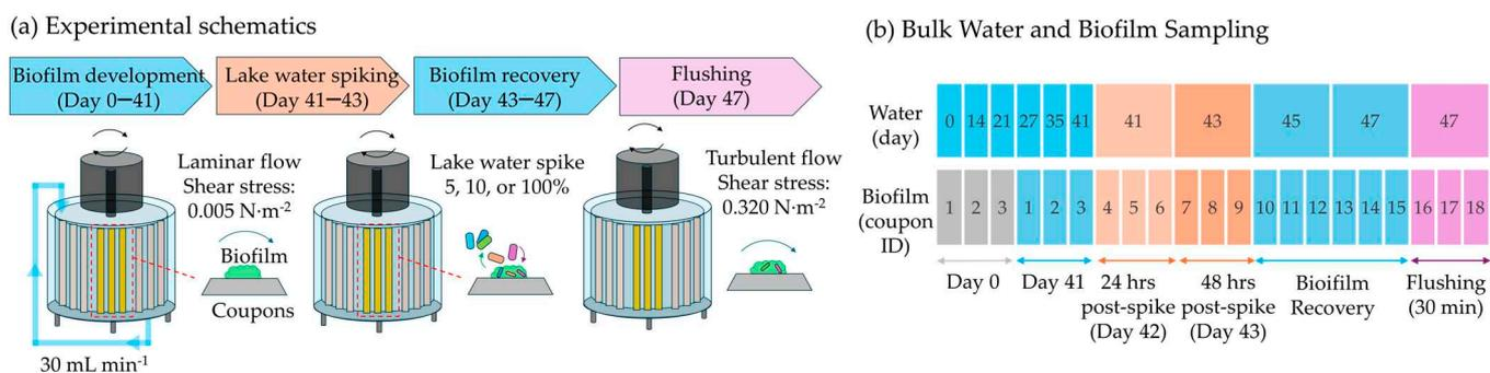
**Figure 1.** Experimental schematics of the annular reactor and biofilm coupon sampling.
