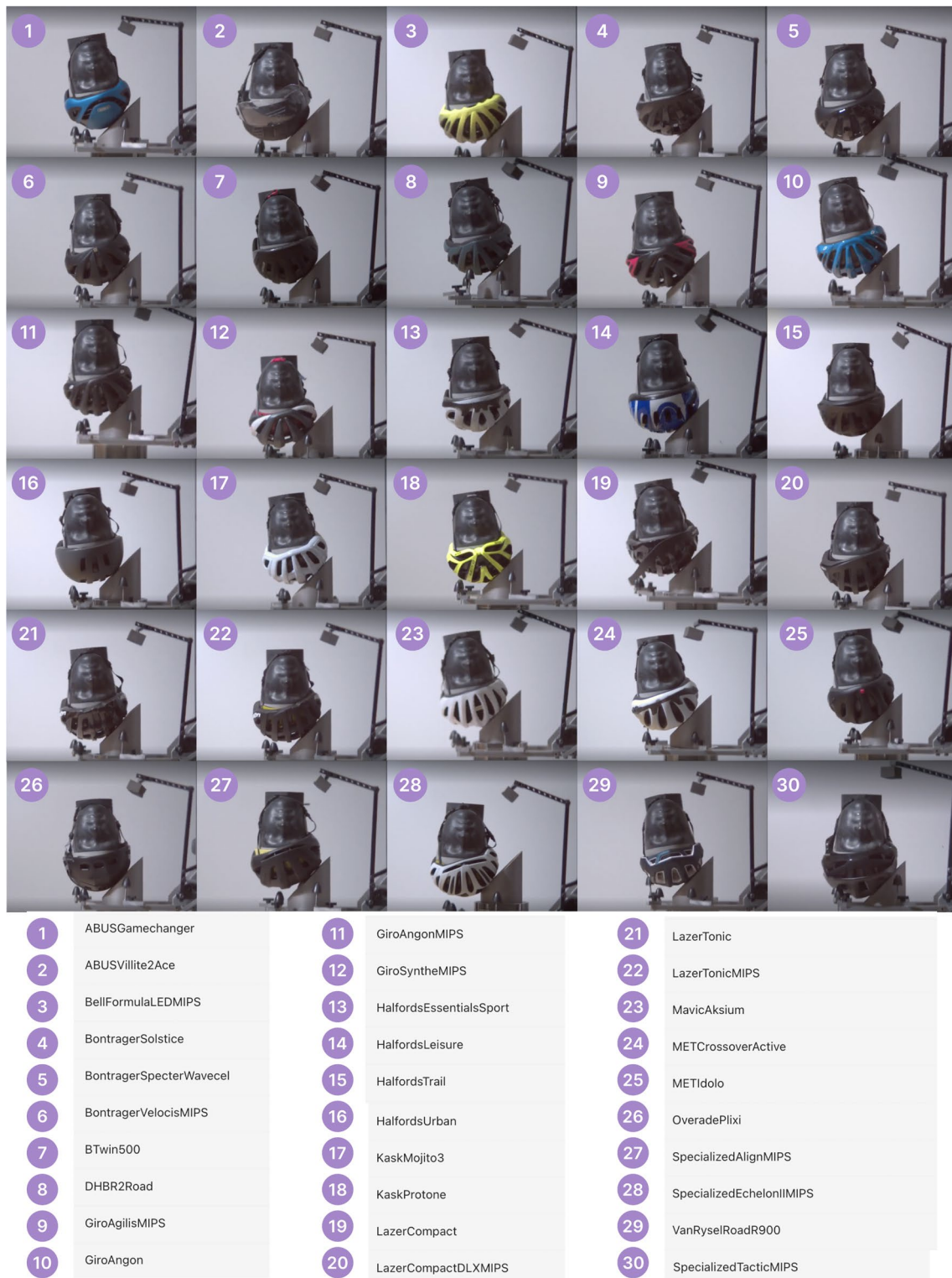
Fig. 2 High-speed footage showing helmet response to impact at 20 ms following the helmet/anvil contact initiation. The pXR configuration is shown
