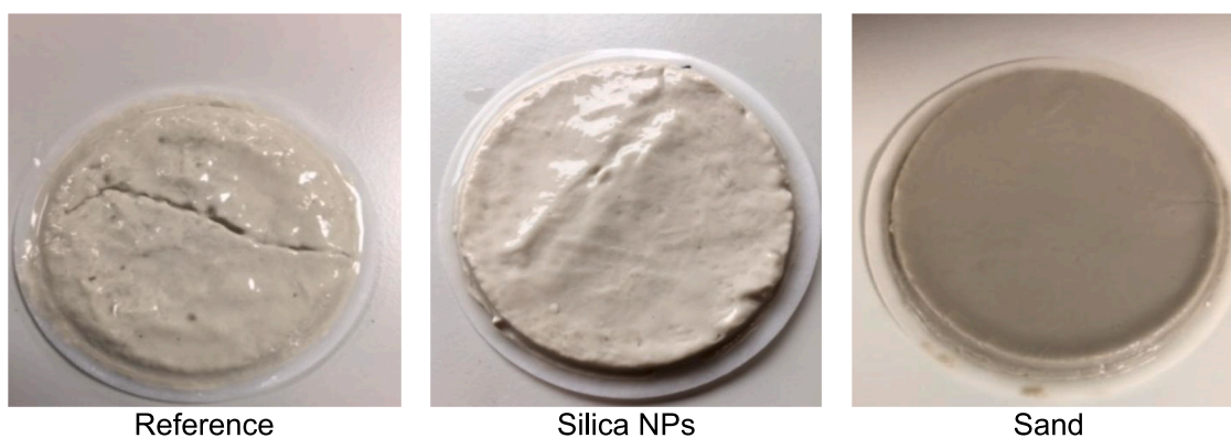
Fig. 9. Mud cakes produced by mud samples containing nano silica and sand under HPHT conditions.
