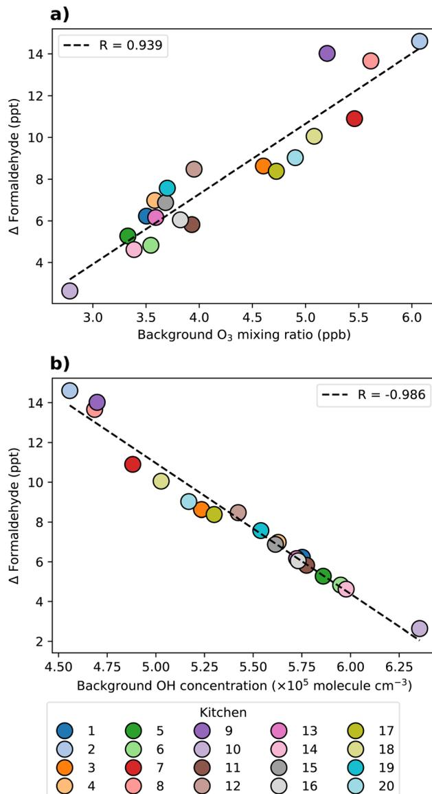
Fig. 8 Correlation of activity-induced changes in formaldehyde with background (a) O<sub>3</sub> and (b) OH concentrations in the basic kitchen permutation simulations. Linear regression analysis was performed to estimate the relationship between variables, with the lines of best fit represented by dashed lines. The Pearson correlation coefficient ( $R$ ) for each plot is displayed in the legend. All the correlations presented are statistically significant ( $p < 0.05$ ).
