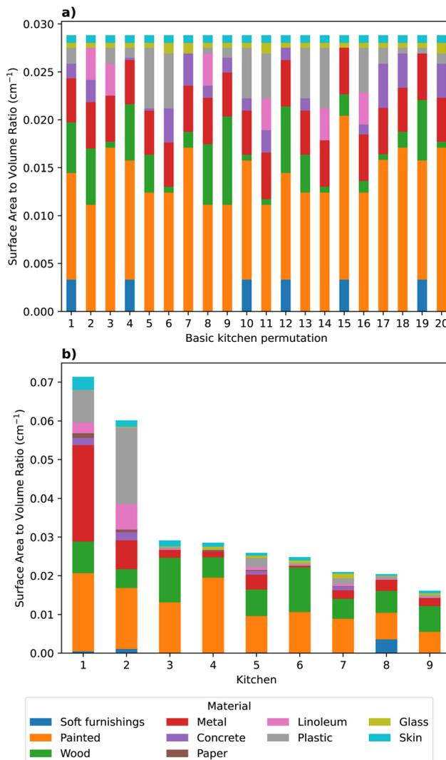
Fig. 2 The material-specific SAVs (cm<sup>-1</sup>) used to initialise the model for the (a) basic kitchen scenario, and (b) real-life kitchen modelling studies.
